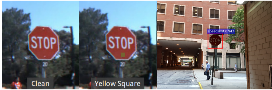
Figure 2.4: Backdoor attack (from [30]). The clean image (left), the clean image with the trigger (middle), and the resulting misclassification (right).
