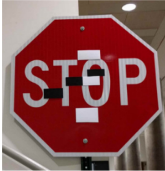
Figure 4.2: Stop sign with adversarial black and white stickers, recognized as a "speed limit 45" road sign, from [59].
