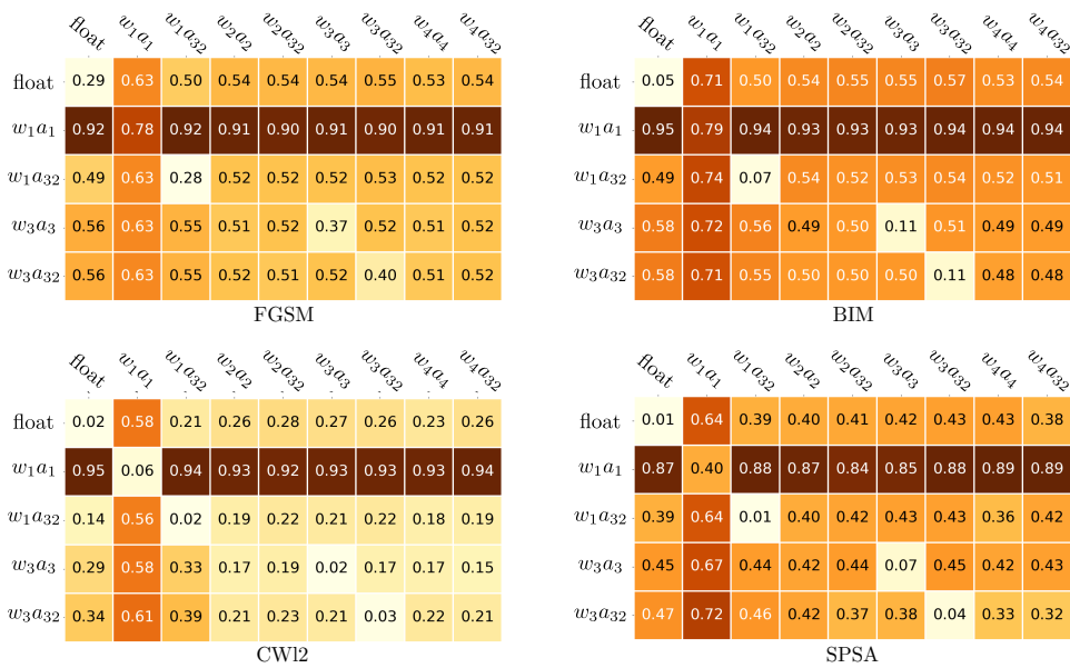
Figure 6.3: Adversarial transferability results for SVHN. Rows are relative to source network and columns to target networks. Values correspond to adversarial accuracy. The lower the value, the more transferability occurs. w_ia_j refers to a model where weights are quantized to i bits and activations to j bits.
