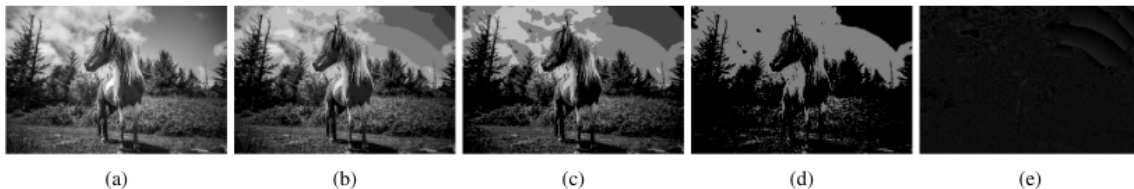
Figure 4.19: Illustration from [172]. (a) Original 8-bit image (b) Weighted sum of (higher) bit planes 7, 6 and 5 (c) Weighted sum of (higher) bit planes 7 and 6 (d) Bit plane 7 - Most significant bit plane (e) Weighted sum of (lower) bit planes 4, 3, 2, 1 and 0
