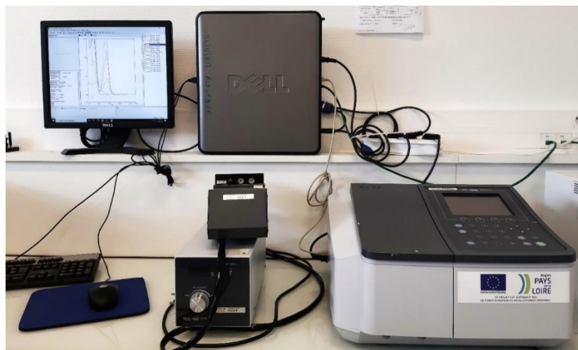
Figure 4.12: UV-1800 (Shimadzu) spectrometer.
