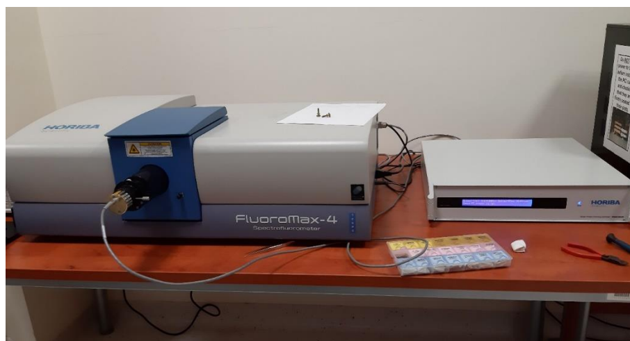
Figure 4.13: Photograph presents spectrofluorometer Horiba FluoroMax-4.
