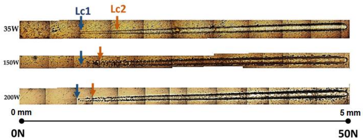
Figure 4.9 Resulting scratch track by increasing load scratch tests for tungsten nitride thin films deposited at different powers and 1 Pa of gas pressure.
