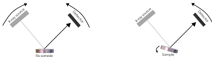
Figure 1.11 Representation of the measurement geometry for the measurements by X-ray diffraction. The image on the left represents the mode \theta – \theta , the image on the right the mode \theta – 2\theta .
