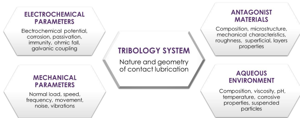
Figure 1.7 Representation of the elements parameters and system characteristics which can influence the response of tribocorrosion processes. Translated from [Richard and Geringer 2019].
