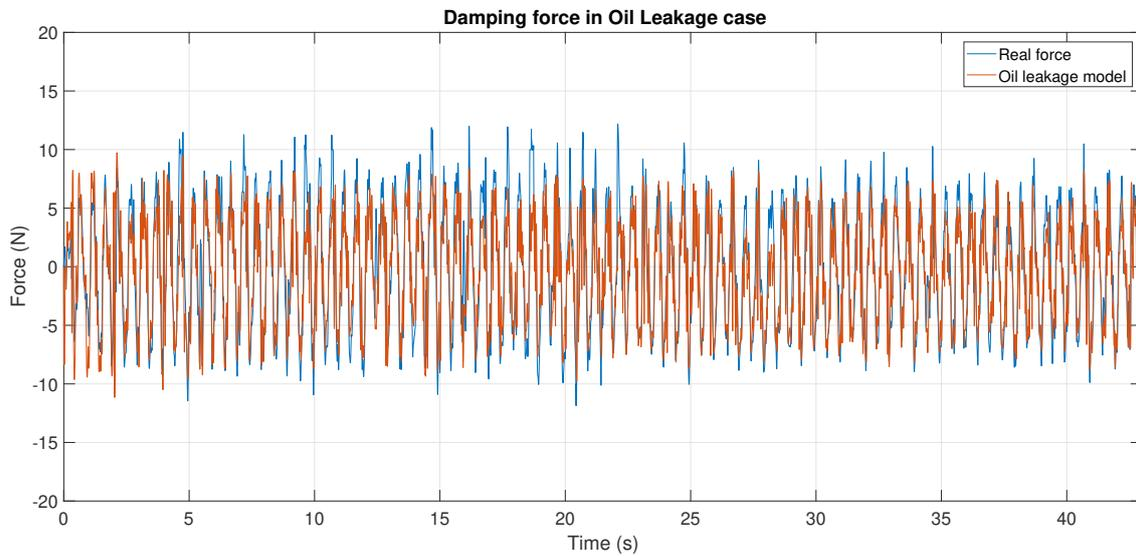
Figure 6.5: Oil leakage: *ER* Damper Force - measurement vs. model
