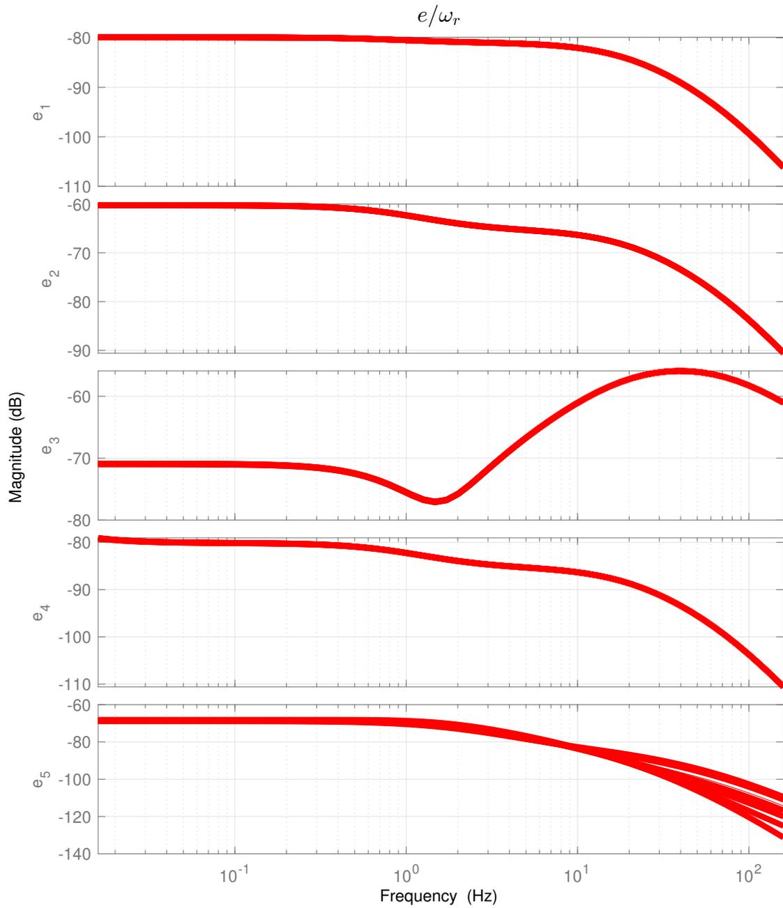
Figure 4.2: Transfer  $\|e/\omega_r\|$ - Bode diagrams of NLPV observer w.r.t. road profile derivative disturbance- gridding method.
