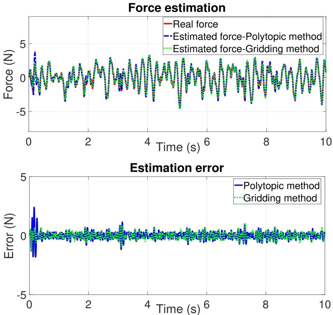
Figure 4.24: Experiment 2: (top) Damper force, (bottom) Estimation error
