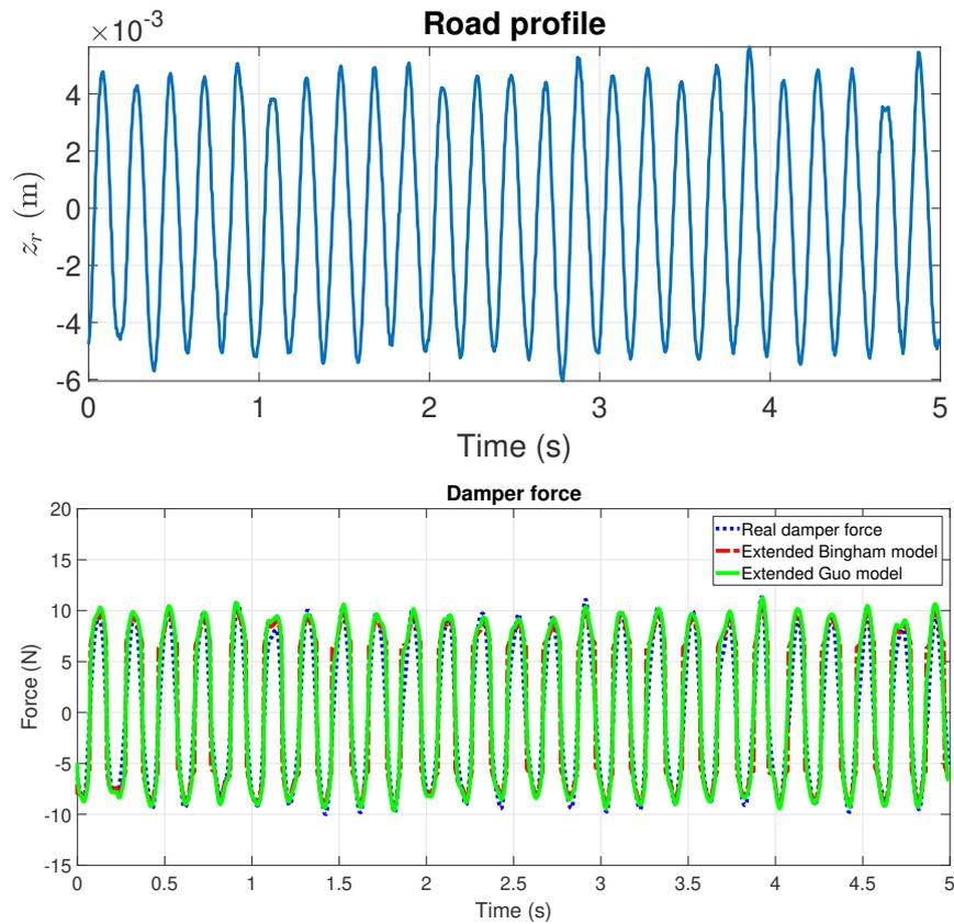
Figure 1.22: Validation Results: (top) Road profile, (bottom) Model-based and Real Force - Sinusoidal Road Profile (Case 3)
