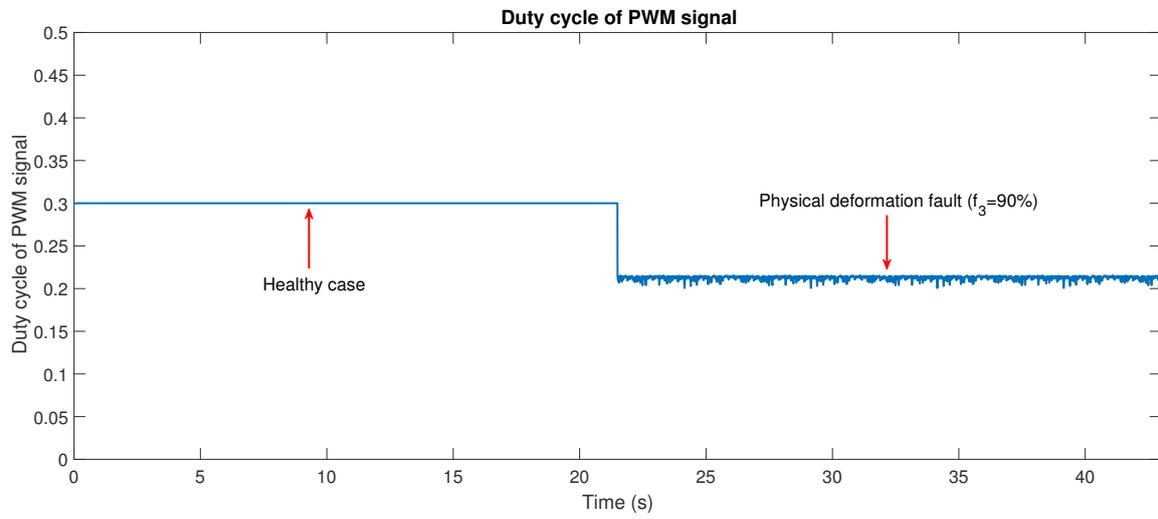
Figure 6.7: Physical deformation: Fault-mimic *PWM* signal
