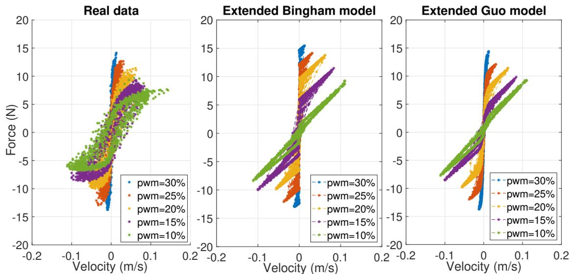
Figure 1.19: Final Model Validation Results: Force vs. Velocity
