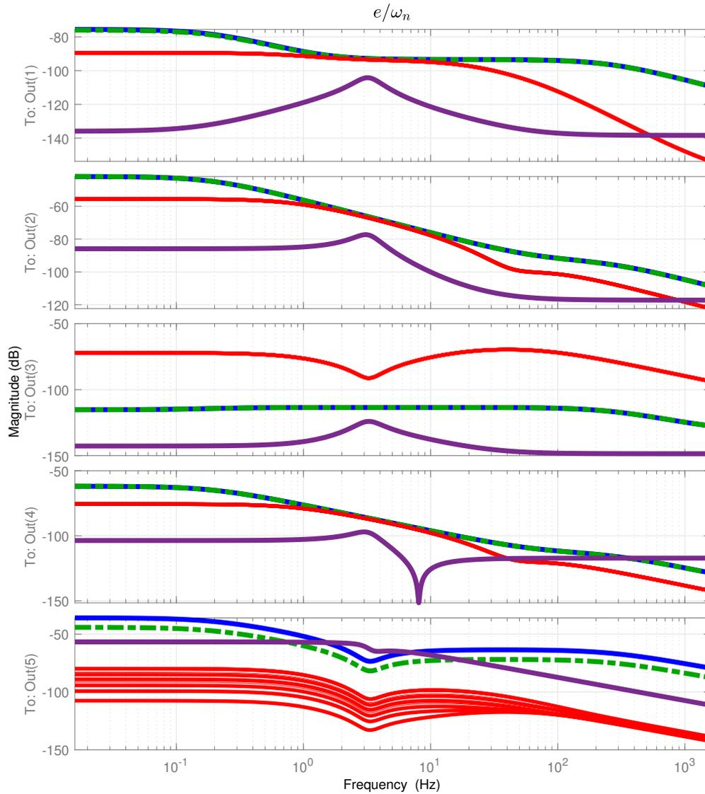
Figure 5.4: Transfer  $\|e/\omega_n\|$ - Bode diagrams of three observers w.r.t. measurement noises- Unified  $H_\infty$  observer (violet line), NLPV polytopic observer (green dash-dot and blue line) and NLPV gridding observer (red line)
