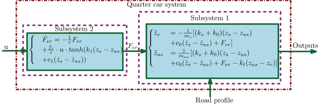
Figure 2.3: System dynamics of quarter vehicle
