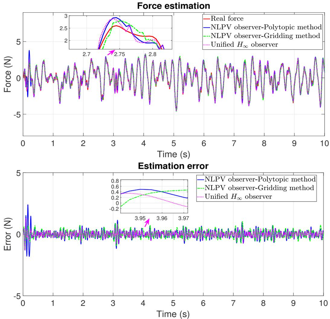
Figure 5.15: Experimental scenario: (above) Damper force, (below) Estimation error
