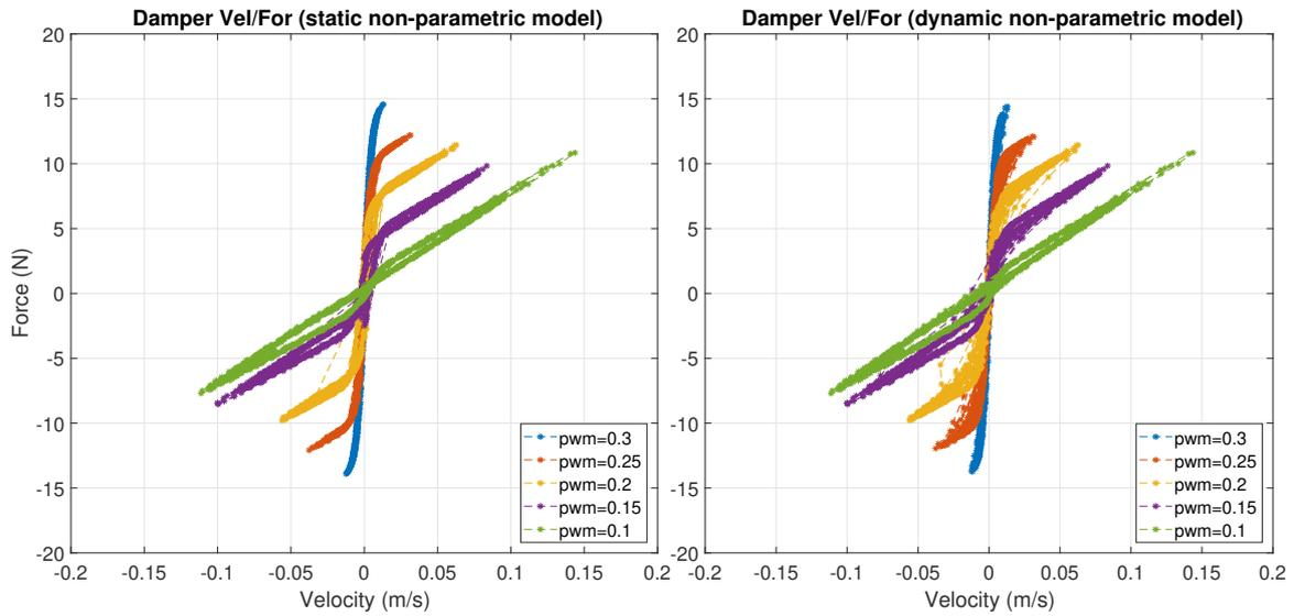
Figure 1.21: Validation Results: Static vs. Dynamical Guo model
