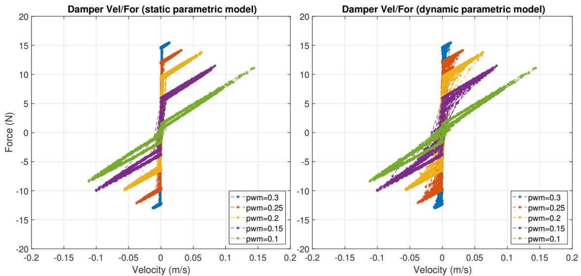
Figure 1.20: Validation Results: Static vs. Dynamical Bingham model
