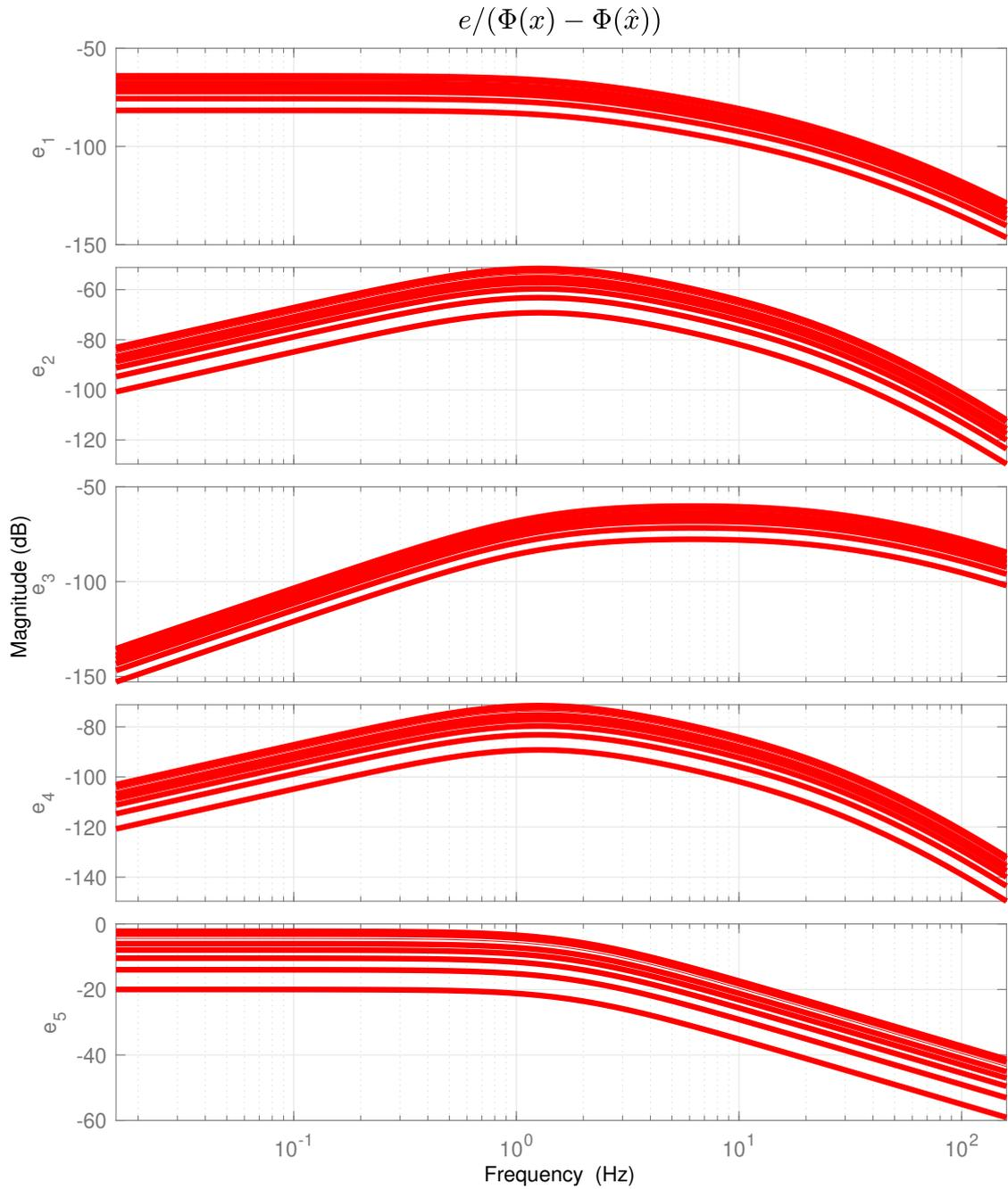
Figure 4.6: Transfer  $\|e/(\Phi(x) - \Phi(\hat{x}))\|$ - Bode diagrams of NLPV observer w.r.t. nonlinearity-gridding method.
