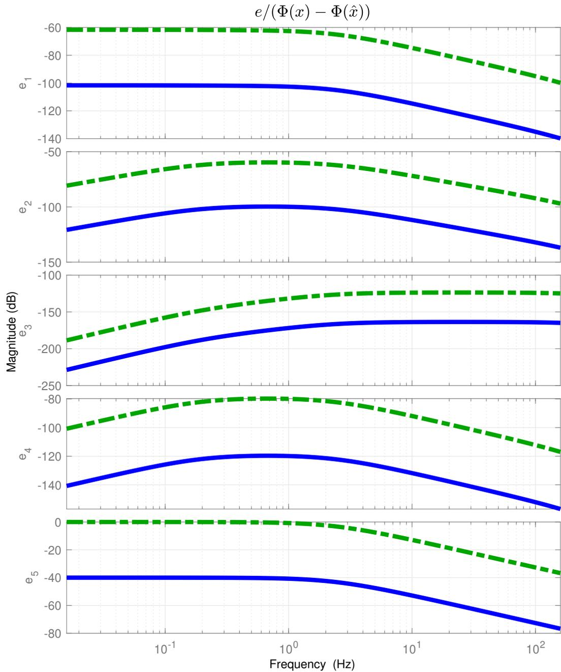
Figure 4.5: Transfer  $\|e/(\Phi(x) - \Phi(\hat{x}))\|$ - Bode diagrams of NLPV observer w.r.t. nonlinearity-polytopic method.
