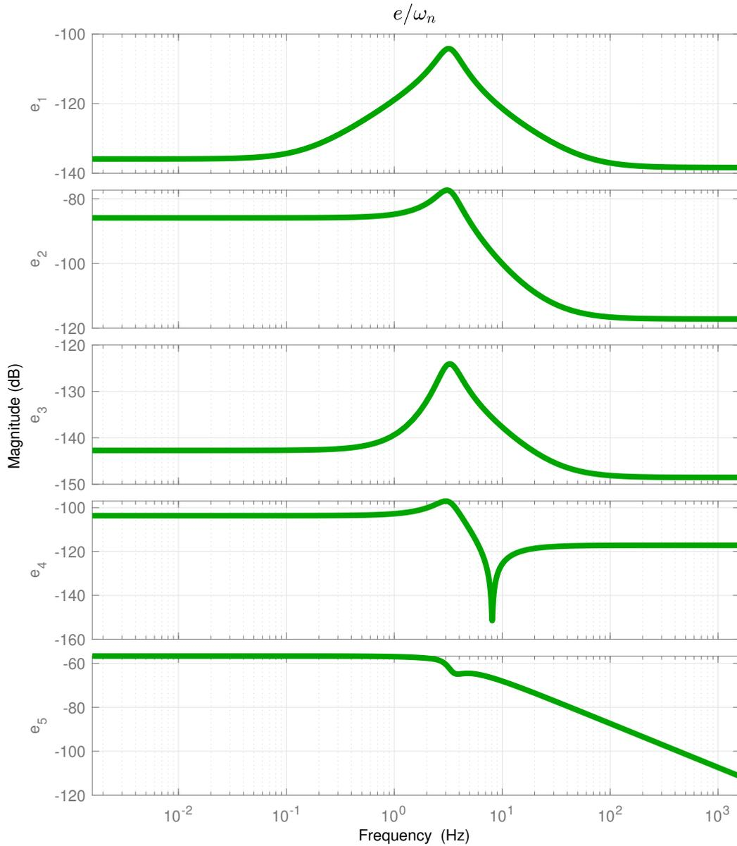
Figure 5.1: Transfer  $\|e/\omega_n\|$ - Bode diagrams of unified  $H_\infty$  observer w.r.t. measurement noises.
