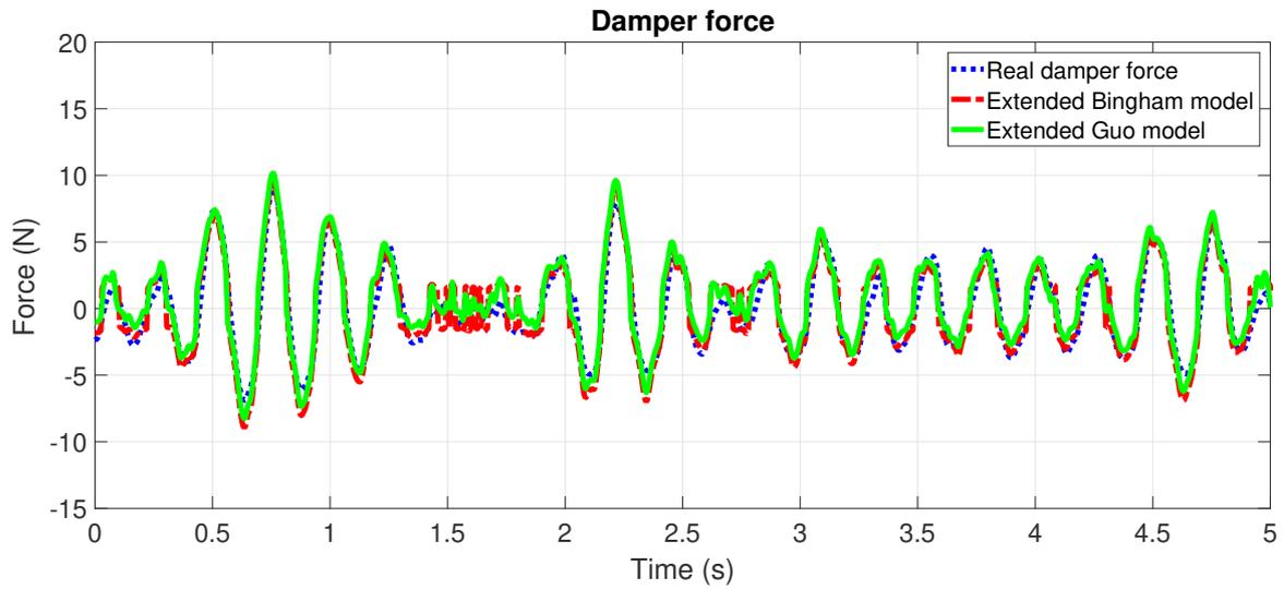
Figure 1.26: Validation Results: Model-based and Real Force - ISO Road Profile (Case 4)
