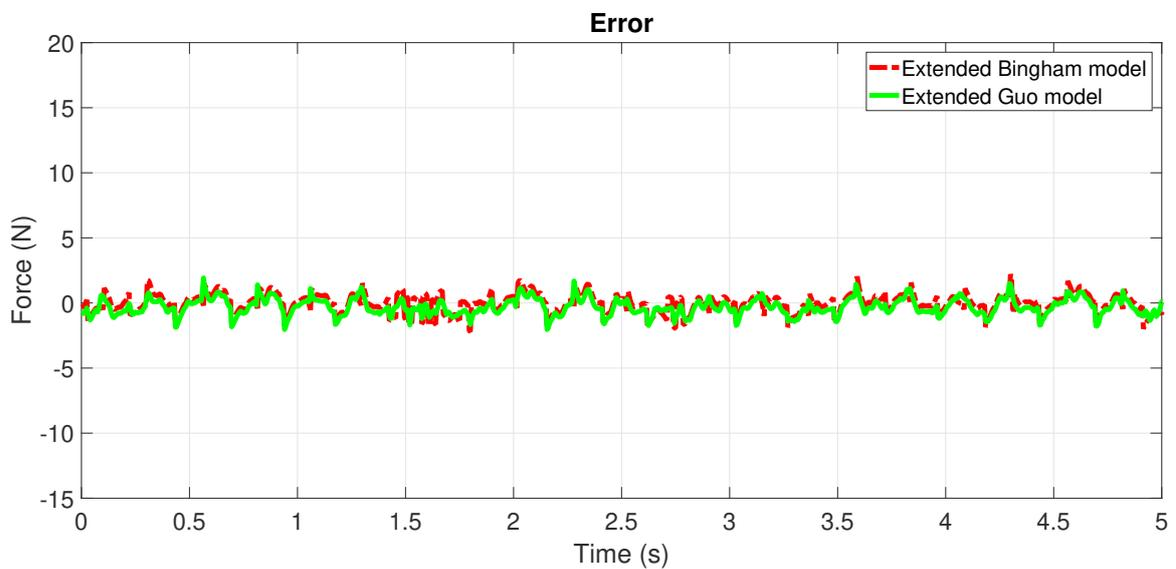
Figure 1.27: Validation Results: Error -ISO Road Profile (Case 4)
