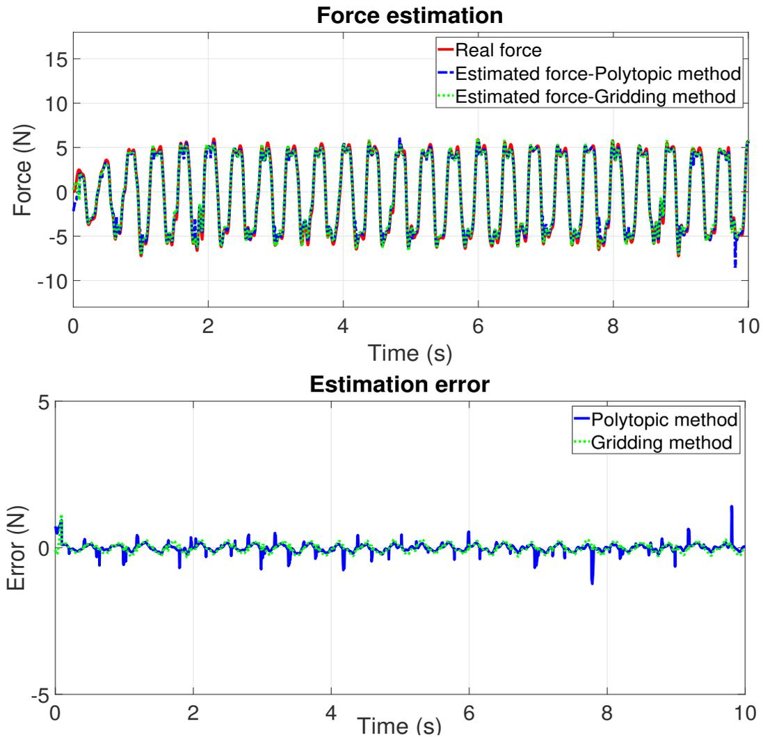
Figure 4.22: Experiment 1: (top) Damper force, (bottom) Estimation error
