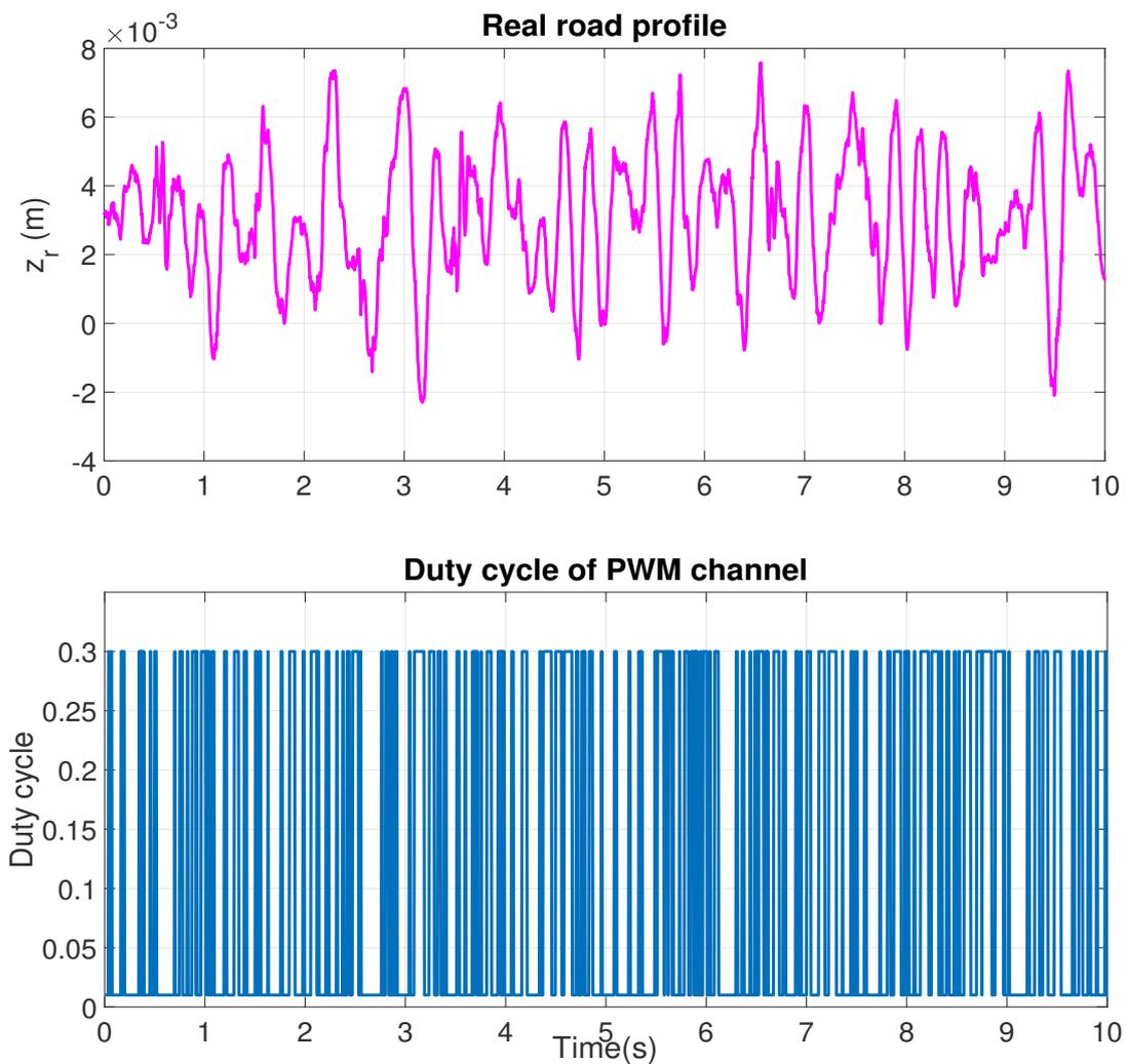
Figure 3.13: Experiment 2: (top) Road profile, (bottom) PWM signal
