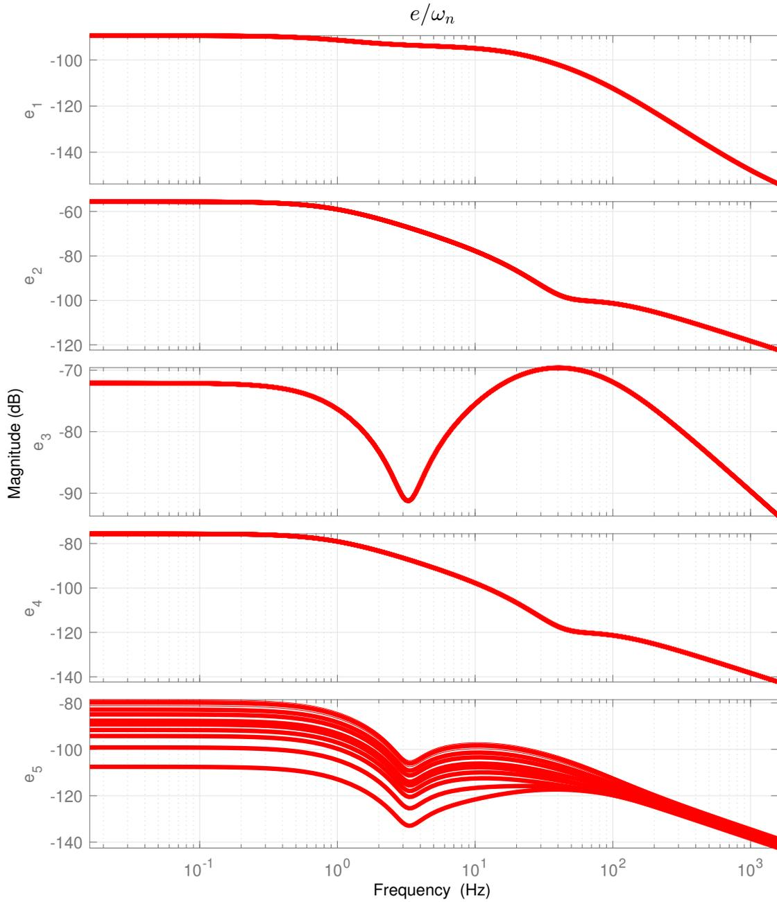
Figure 4.4: Transfer  $\|e/\omega_n\|$ - Bode diagrams of NLPV observer w.r.t. measurement noises-gridding method.
