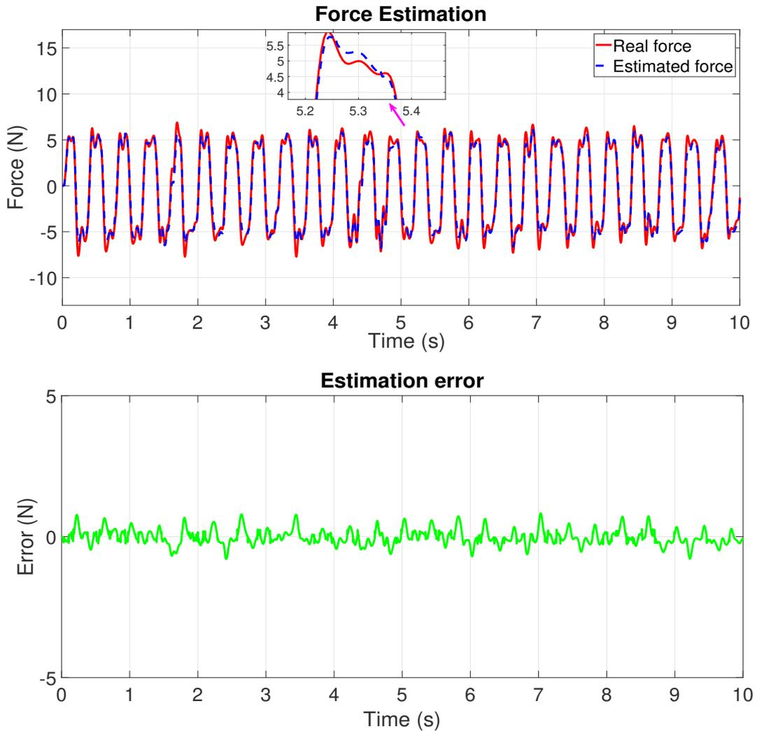
Figure 3.12: Experiment 1: (top) Damper force, (bottom) Estimation error
