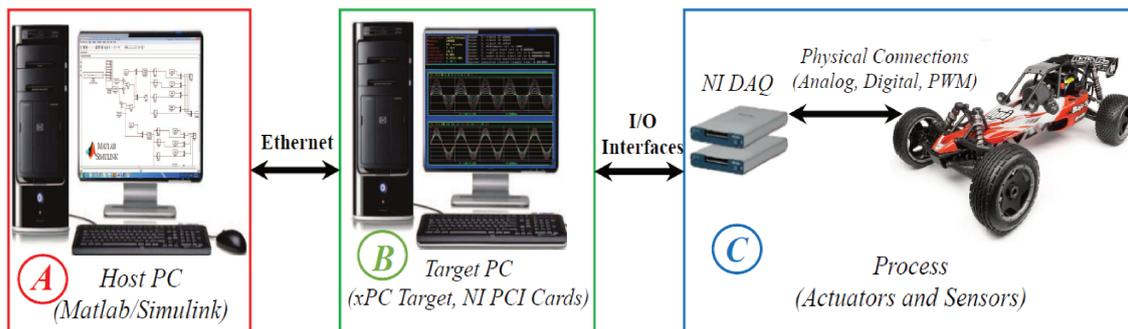
Figure 1.4: Schematic of INOVE experimental platform [Tudón-Martínez et al. 2015]
