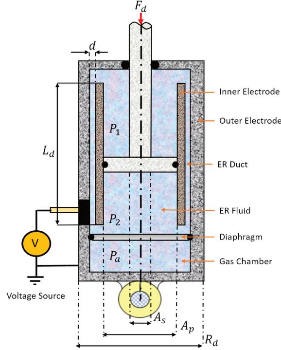
Figure 1.6: Schematic Representation of an ER Damper, adapted from [Choi and Han 2003]
