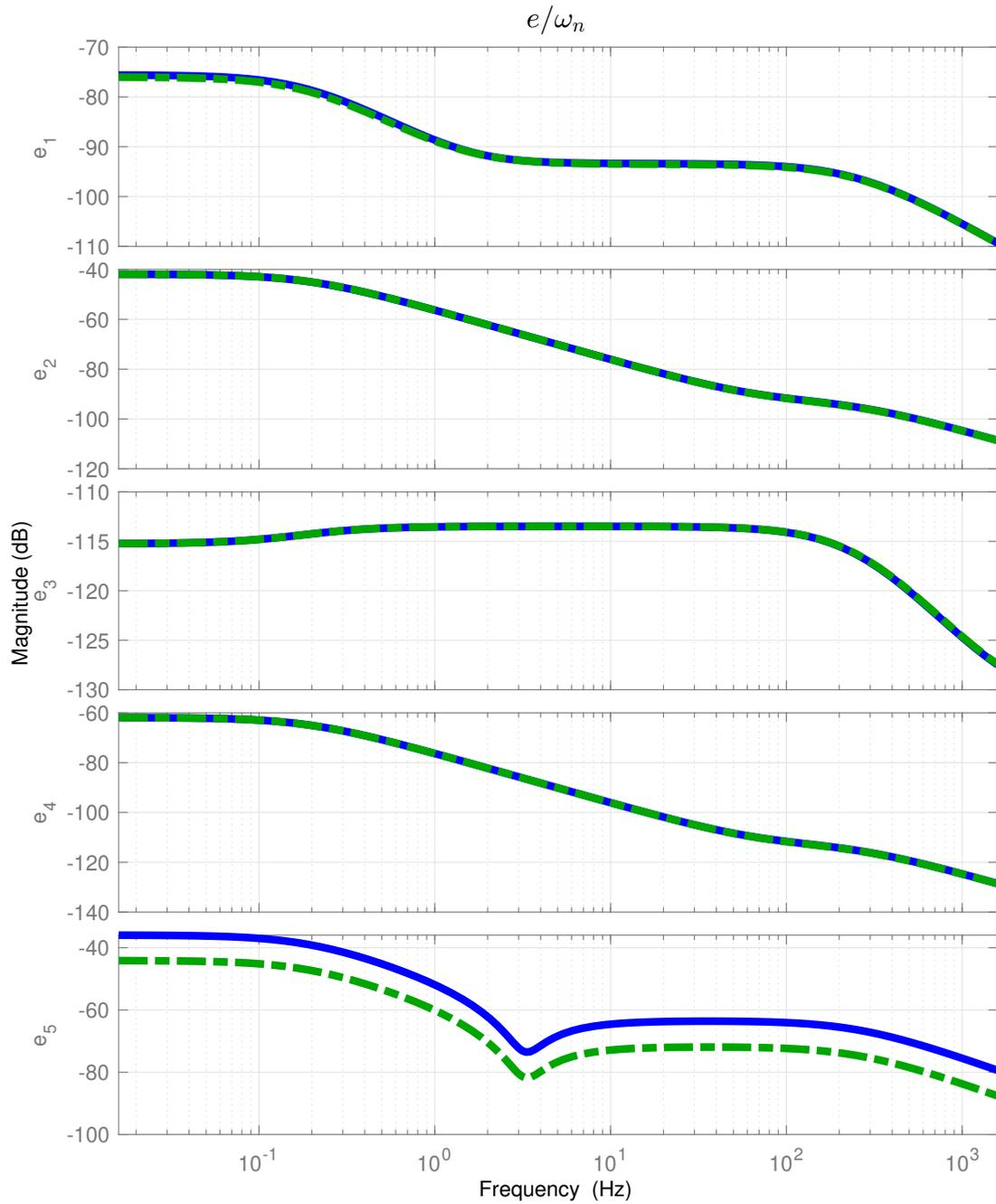
Figure 4.3: Transfer  $\|e/\omega_n\|$ - Bode diagrams of NLPV observer w.r.t. measurement noises- polytopic method .
