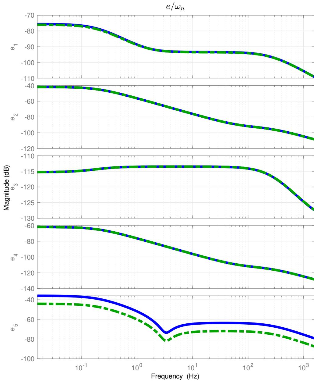
Figure 5.2: Transfer  $\|e/\omega_n\|$ - Bode diagrams of NLPV observer w.r.t. measurement noises-polytopic method .
