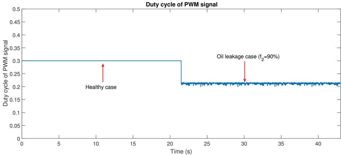
Figure 6.4: Oil leakage: Fault-mimic *PWM* signal
