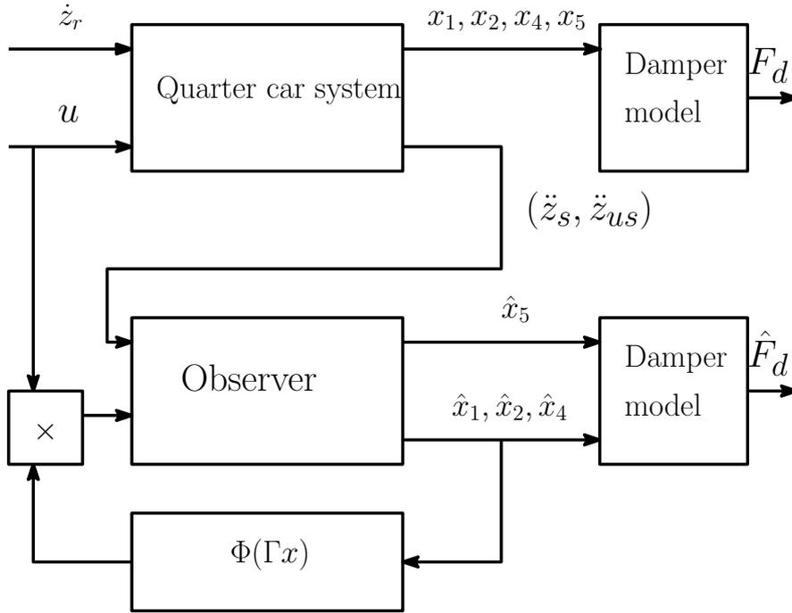
Figure 3.3: Block diagram for simulation of the observer
