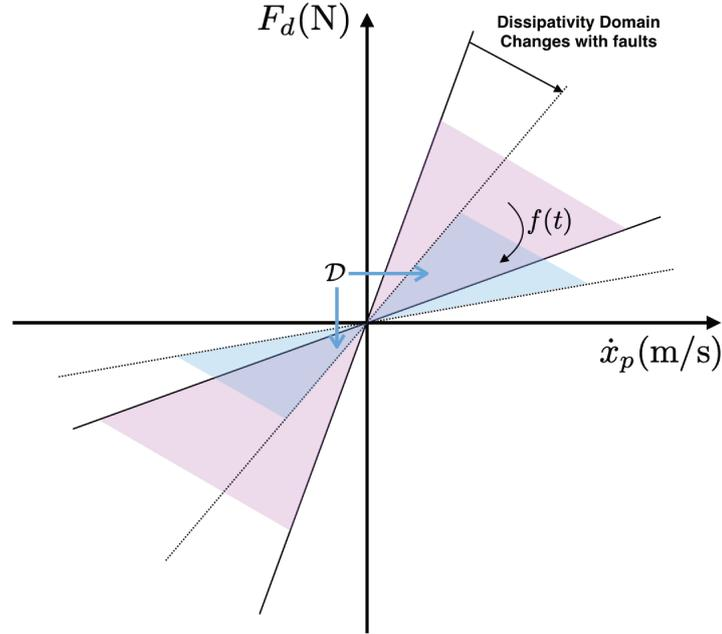
Figure 6.10: The ideal dissipative force domain  $\mathcal{D}_f$  in presence of fault
