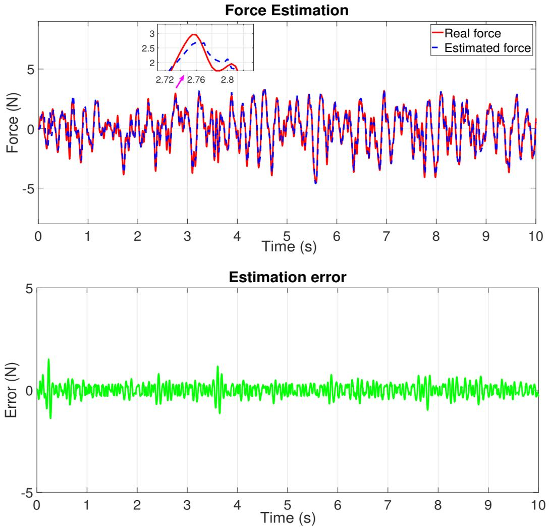
Figure 3.14: Experiment 2: (top) Damper force, (bottom) Estimation error
