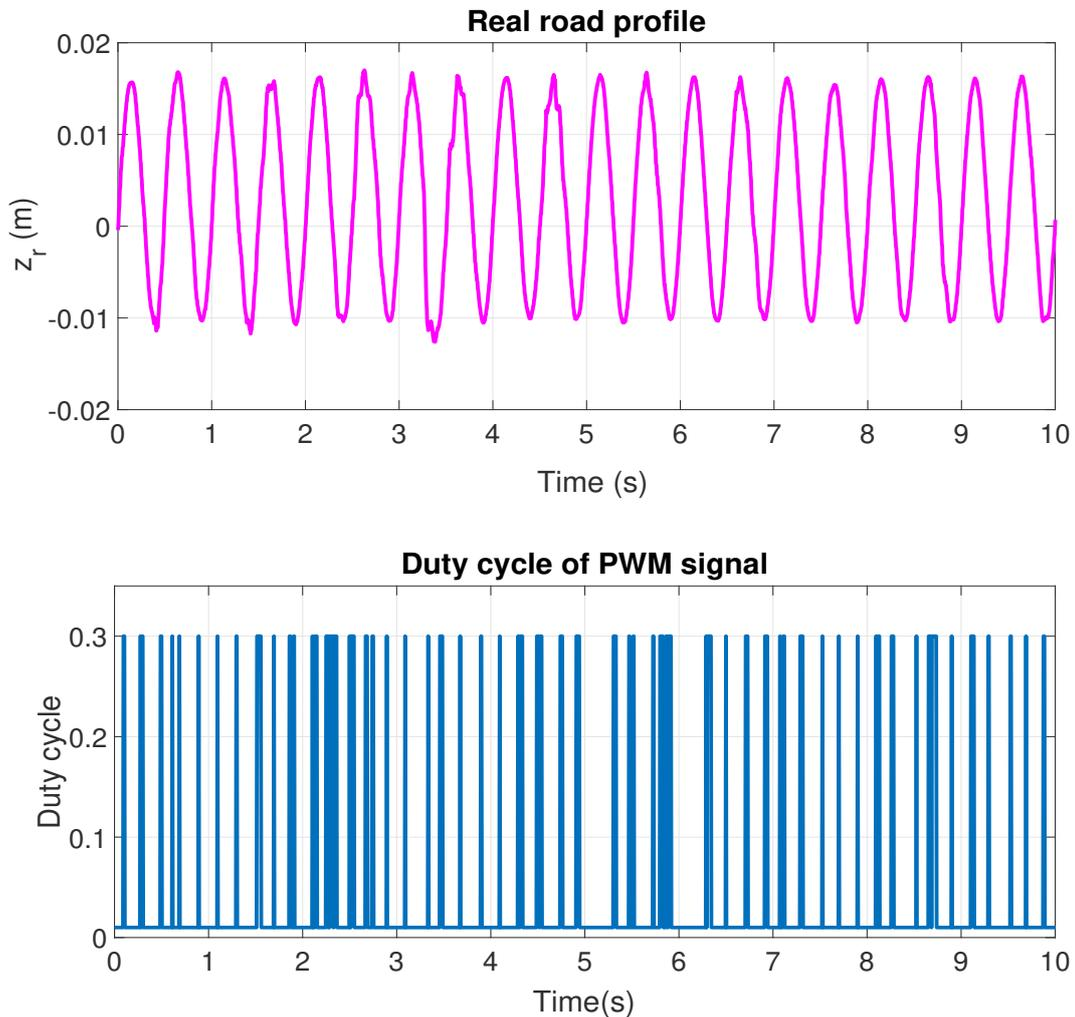
Figure 3.11: Experiment 1: (top) Road profile, (bottom) PWM signal
