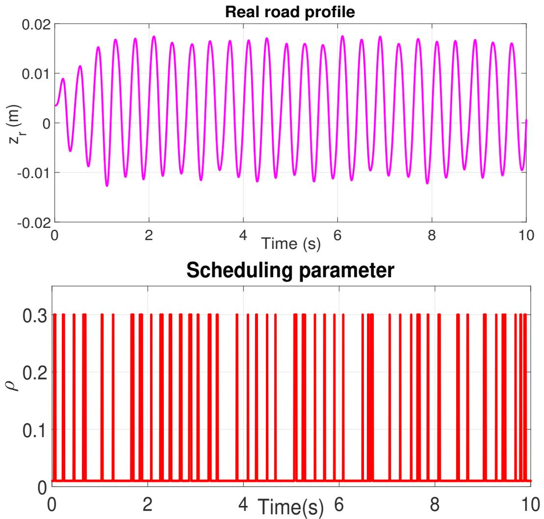
Figure 4.21: Experiment 1: (top) Road profile, (bottom) Scheduling parameter
