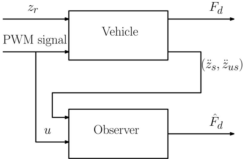
Figure 3.10: Block diagram for implementation of the observer
