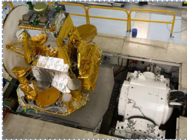
Figure 1-2 Satellite on the vibration testing facility at Thales Alenia Space
