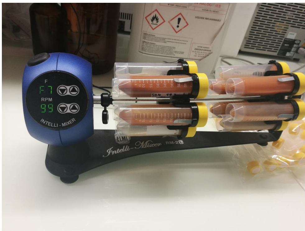
Figure 21 : A photo showing the rotating shaker used during the exchangeable phase extraction ( 2 \times 1\text{h} ).
