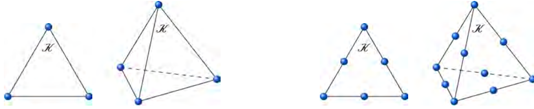
(a) Degrees of freedom for a continuous piecewise linear finite element space P_1 .
