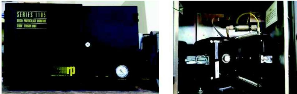
Figure 5. Tapered Element Oscillating Microbalance (TEOM)
