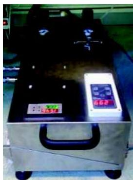
Figure 3. Pegasor Particle Sensor (PPS)
