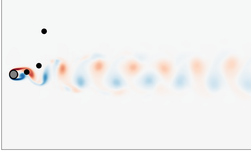
Figure 5.1: Vorticity field for a flow around a cylinder, Re = 200 , selection of three random points in the domain.
