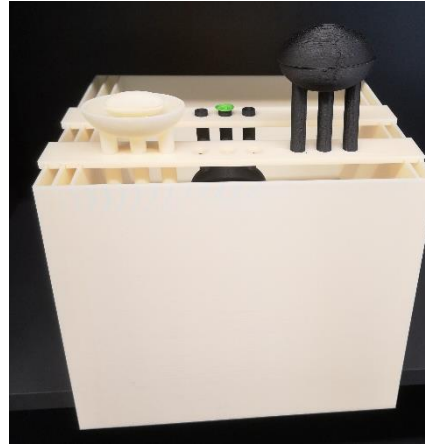
Figure 2.34: First prototype of a multilayer abdomen with the ablated liver cavity
