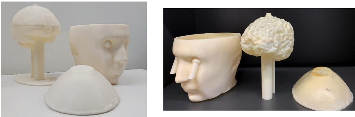
Figure 2.24: Head phantoms including on Right: two cavities and on left: three cavities with a circumvolution's brain.
