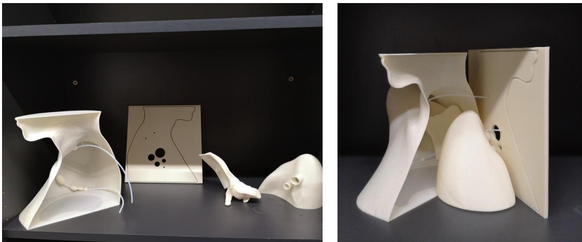
Figure 2.30: 3D printed axillary phantom based on online phantom library.
