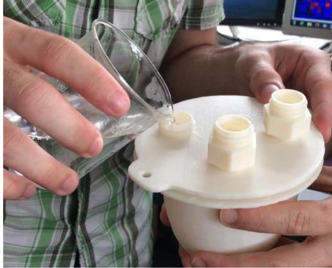
Figure 2.1: Filling the cavity, which represents human breast with mixture mimicking breast tissues.
