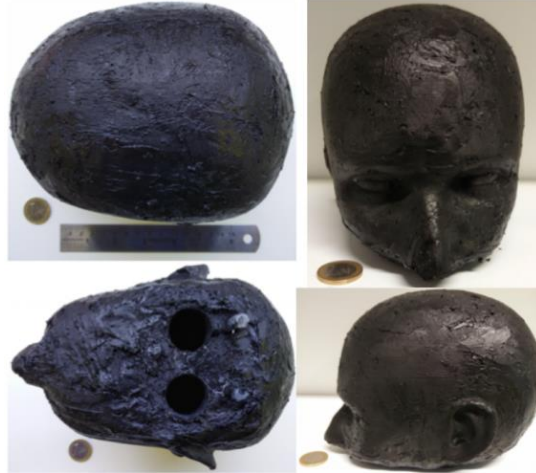
Figure 2.26: Photograph of the fabricated dielectrically and anatomically realistic C-black head phantom [McDermott et al. , 2017].
