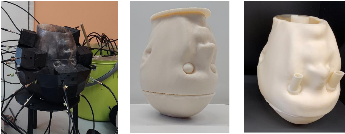
Figure 2.23: Upside down head phantoms, prepared for the POLITO microwave imaging system.
