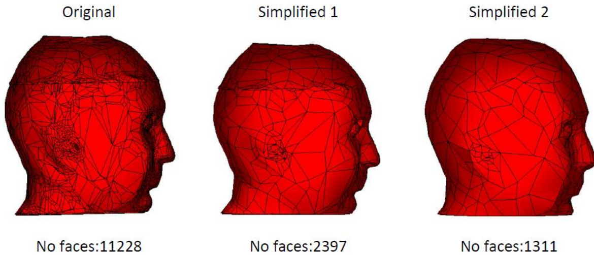
Figure 3.13: Using WIPL-D for re-meshing the head phantom, preparing it for new simulations in WIPL-D.
