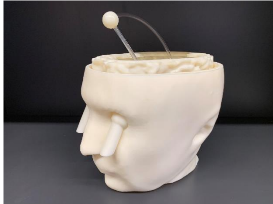
Figure 2.25: A sphere located in the head phantom as a stroke.
