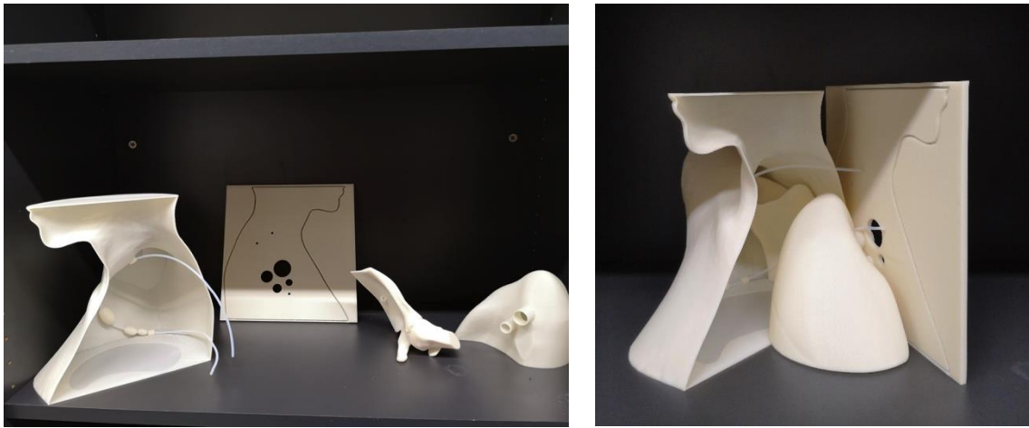
Figure 2.30: 3D printed axillary phantom based on online phantom library.
