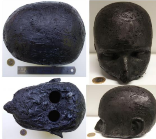
Figure 2.26: Photograph of the fabricated dielectrically and anatomically realistic C-black head phantom [McDermott et al. , 2017].
