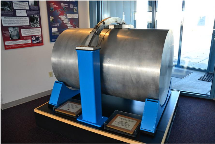
Figure 1.4: A Weber bar, exposed at the LIGO Handford observatory. It consists of an aluminium bar with a piezo-electric readout on the top of the bar. Image taken from [81].
