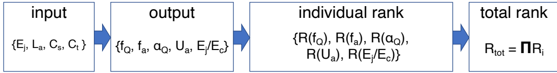
Figure 2.1: Process of ranking the set of input parameters. First, we calculate a set of output parameters related to the input parameters, based on equations 1.1.4. After ranking each of the output parameters (spectroscopic values) individually, we multiply them to calculate a total rank. Our goal is to maximize the product in the optimization algorithm.
