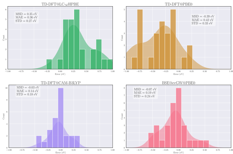
Figure 3.12: Error distribution of TD-DFT calculations for 30 optical transitions on 17 molecular compounds against the theoretical best estimate for three different exchange-correlation functionals. (top left) LC- \omega HPBE, (top right) PBE0, (bottom left) CAM-B3LYP, (bottom right) BSE@evGW@PBE0.
