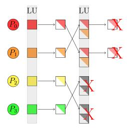
Figure 4.6: FT-TSLU example with t = 4 processes, showing two failures in the same branch at the middle step.
