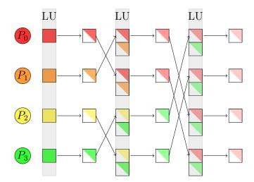
Figure 4.2: FT-TSLU failure-free example with t=4 processes. Gray bar represents the moment when a LU factorization is performed.
