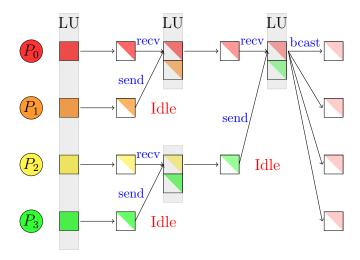
Figure 4.1: TSLU failure-free example with t = 4 processes. Gray bar represents the moment when a LU factorization is performed.
