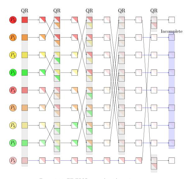
Figure 8.11: FT-TSQR example with t = 9 processes.
