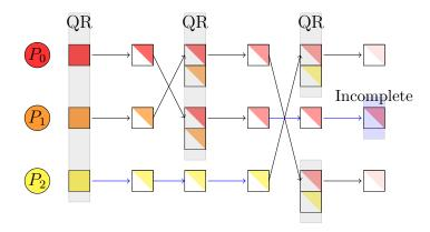
Figure 8.9: FT-TSQR example with t = 3 processes.
