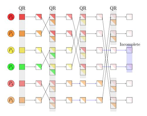
Figure 8.12: FT-TSQR example with t = 6 processes.
