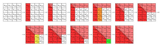
Figure 4.10: Square matrix partition by sub-blocks, panels selection and trailing matrix update example.
