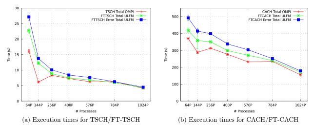
Figure B.9: Total times obtained in (FT-)TSCH/(FT-)CACH algorithms (input:  $64k \times 64k$ ).
