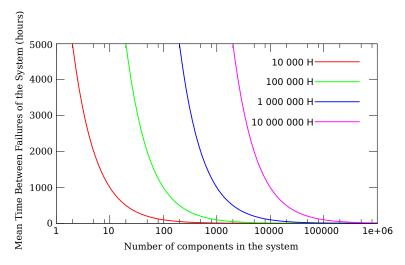
Figure 1.1: Mean Time Between Failures example
