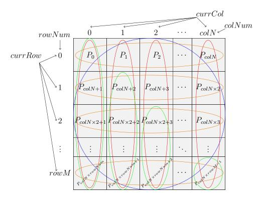
Figure 8.8: Communication-Avoiding grid partitioning description: red=column communicators, orange=row communicators, green=panel communicators, blue=global communicator; rowM = M - 1, colN = N - 1,  $\{currRow, rowNum\} \in [0, rowM]$ ,  $\{currCol, colNum\} \in [0, colN]$
