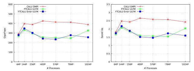
(a) Maximal throughput reached in CALU/FT-CALU(b) Maximal speed-up reached in CALU/FT-CALU executions
