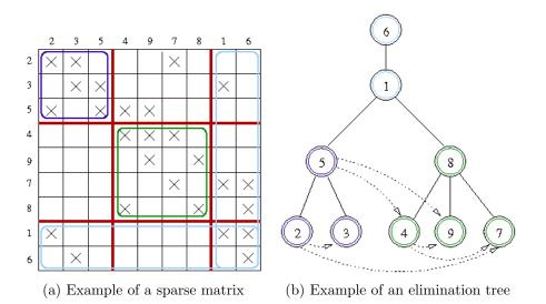
Figure 10.1: Example of a sparse matrix with an elimination tree.
