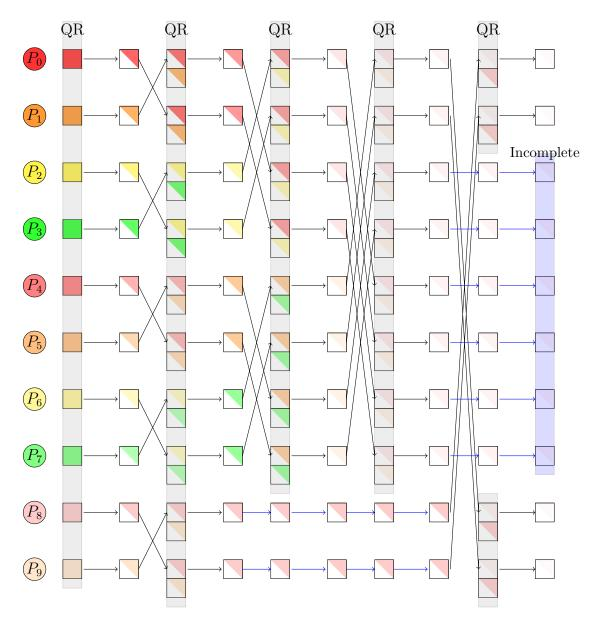
Figure 8.13: FT-TSQR example with t = 10 processes.
