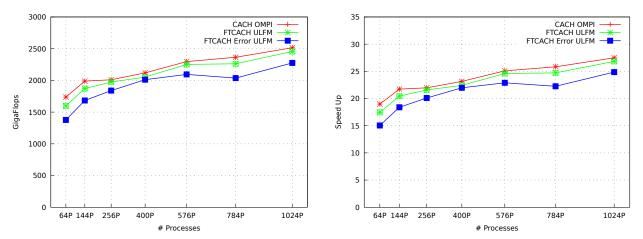
(a) Maximal throughput reached in CACH/FT-CACH(b) Maximal speed-up reached in CACH/FT-CACH executions ecutions
