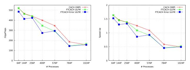
(a) Maximal throughput reached in CACH/FT-CACH(b) Maximal speed-up reached in CACH/FT-CACH executions ecutions  $\frac{1}{2}$
