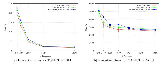
Figure 9.1: Total times obtained in (FT-)TSLU/(FT-)CALU algorithms (input:  $100k \times 100k$ ).
