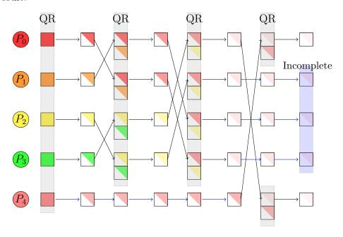
Figure 8.10: FT-TSQR example with t = 5 processes.
