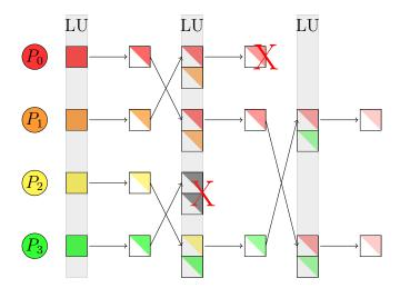
Figure 4.4: FT-TSLU example with t = 4 processes, showing one failure at the middle step.
