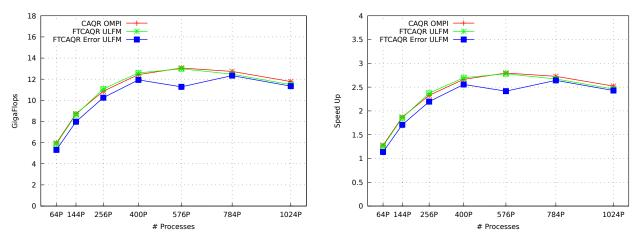
(a) Maximal throughput reached in CAQR/FT-CAQR(b) Maximal speed-up reached in CAQR/FT-CAQR executions
