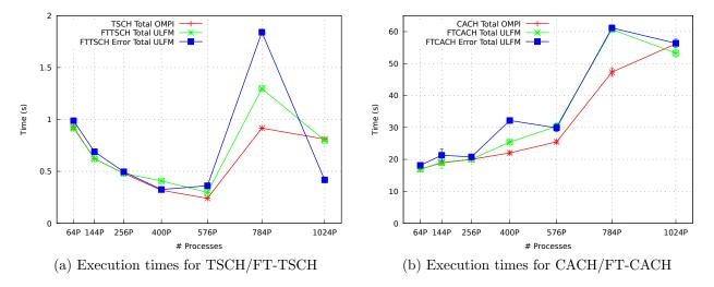
Figure B.5: Total times obtained in (FT-)TSCH/(FT-)CACH algorithms (input:  $16k \times 16k$ ).
