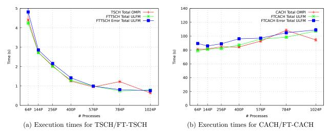
Figure B.7: Total times obtained in (FT-)TSCH/(FT-)CACH algorithms (input:  $32k \times 32k$ ).
