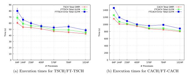
Figure 9.7: Total times obtained in (FT-)TSCH/(FT-)CACH algorithms (input:  $100k \times 100k$ ).
