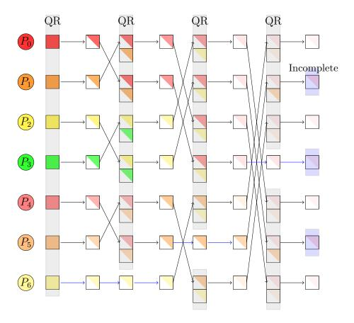
Figure 8.14: FT-TSQR example with t = 7 processes.
