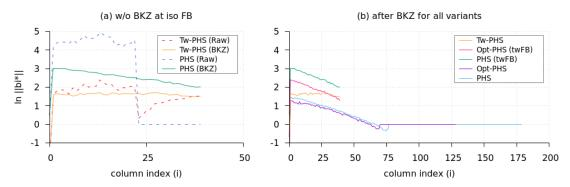
FIGURE 3.22 – Log-S-unit lattices for  $\mathbb{Q}(z_{47})$ , Gram-Schmidt log norms: (a) before and after BKZ<sub>40</sub> reduction at iso factor base  $\mathcal{A}_{\mathsf{tw-FB}}(K)$  for  $L_{\mathsf{tw}}$  and  $L_{\mathsf{phs}}^{\scriptscriptstyle{(0)}}$ ; (b) after BKZ<sub>40</sub> reduction for all variants  $L_{\mathsf{tw}}$ ,  $L_{\mathsf{opt}}^{\scriptscriptstyle{(0)}}$ ,  $L_{\mathsf{opt}}$  and  $L_{\mathsf{phs}}$ .
