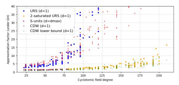
FIGURE 5.3 – Approximation factors, with Gaussian Heuristic, reached by Twisted-PHS for cyclotomic fields of degree up to 210, on lattices  $L_{\sf urs}$ ,  $L_{\sf sat}$  and  $L_{\sf su}$ .
