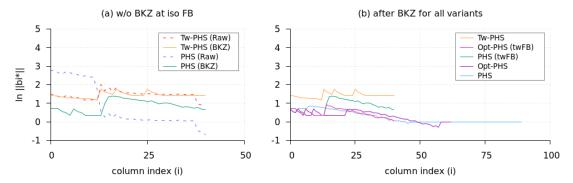
FIGURE 3.7 – Log-S-unit lattices for  $\mathbb{Q}(\zeta_{29})$ , Gram-Schmidt log norms: (a) before and after BKZ<sub>40</sub> reduction at iso factor base  $\mathcal{A}_{\mathsf{tw-FB}}(K)$  for  $L_{\mathsf{tw}}$  and  $L_{\mathsf{phs}}^{(0)}$ ; (b) after BKZ<sub>40</sub> reduction for all variants  $L_{\mathsf{tw}}$ ,  $L_{\mathsf{opt}}^{(0)}$ ,  $L_{\mathsf{phs}}^{(0)}$ ,  $L_{\mathsf{opt}}$  and  $L_{\mathsf{phs}}$ .
