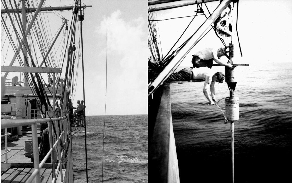
Figures 4 and 5: Kullenberg's piston corer onboard the Swedish vessel Albatross . The left image depicts the instrument in vertical, waiting to be descended. On the right, two oceanographers are hinging the samples (source: WHOI Online Repository, 1949).
