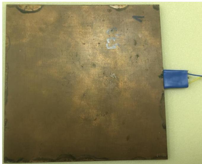
Fig. 3.6 Heat flux sensor
