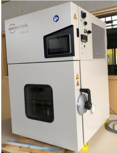
Fig. 3.4 Climatic chamber (LabEvent L C/64/40/3)
