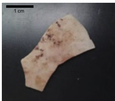
Figure I.2. Plastic debris used to produce the e-NPs suspension, showing brown algae residue on its surface
