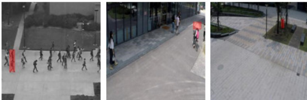
FIGURE 4.41 – Several imperfect cases of anomaly localisations affected by Mask R-CNN detector. Left : Too large bounding box ; Middle : Too small box ; Right : Wrong object. Best viewed in color.
