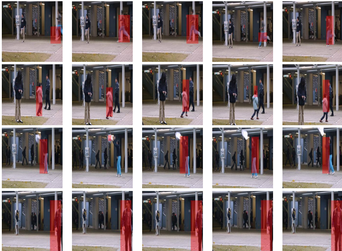
FIGURE 4.36 – Qualitative results of single abnormal object localization on Avenue dataset. Each row represents a type of abnormality. From the top row to the bottom row : running, dancing, throwing object, moving to wrong direction. We can exactly detect the abnormal object in every frame. Due to the drawback of Mask R-CNN, the bounding boxes are not perfect in some cases, e.g. 4 th image of the first and second rows, 2 nd image of the third row.
