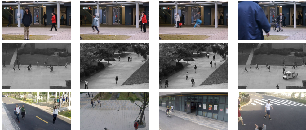
FIGURE 4.5 – Illustration of several samples in CUHK-Avenue dataset [58], USCD-Pedestrian datasets [66] and ShanghaiTech dataset [53]. First row : Avenue dataset. Second row : Pedestrian dataset. Third row : ShanghaiTech dataset. ShanghaiTech is more challenging than other due to multiple captured views and flexible abnormal samples.
