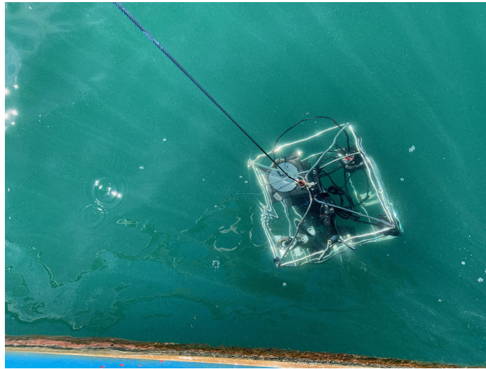
FIGURE 1.2: Measuring equipment being deployed in the English Channel from the CNRS research vessel Sepia (based in Boulogne-sur-Mer) during a campaign to which the author participated in 2020. The objective of the campaign was to sample temperature, salinity, chlorophyll, PAR (radiation), ocean kinetic energy dissipation rate and velocity in multiple locations. Unfortunately due to the restricted number of sampling days under the pandemic of 2020/2021 the data obtained was insufficient for analysis.
