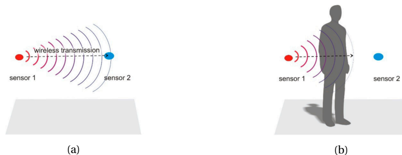
FIGURE 2.2 – Illustration of body shadowing on wireless transmission between sensors : (a) Line-of-sight, successful transmission; (b) body shadowing that affects transmission (Taken from Januszkiewicz [5])
