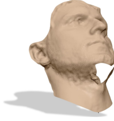
Figure 2.4: Example of scanned mesh with a hole caused by light reflections on the beard.
