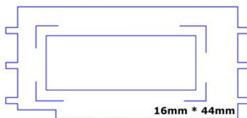
Figure 2.13: Design of the frame to be cut.
