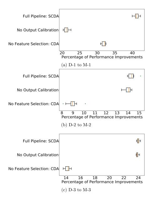
Figure 4.6: The log-loss improvements of Kaggle fraud detection tasks with LGB models. "Full Pipeline: SCDA" represents our adaptation model with full 3 steps (see Figure 4.1). Whereas "No Output Calibration" skips the first step, and "No Feature Selection: CDA" skips the third step.
