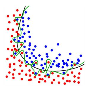
Figure 2.1: Red points and blue points represent training examples of two classes. The green curve is an overfitted model, while the black curve is a regularized one (Chabacano 2008).<sup>1</sup>
