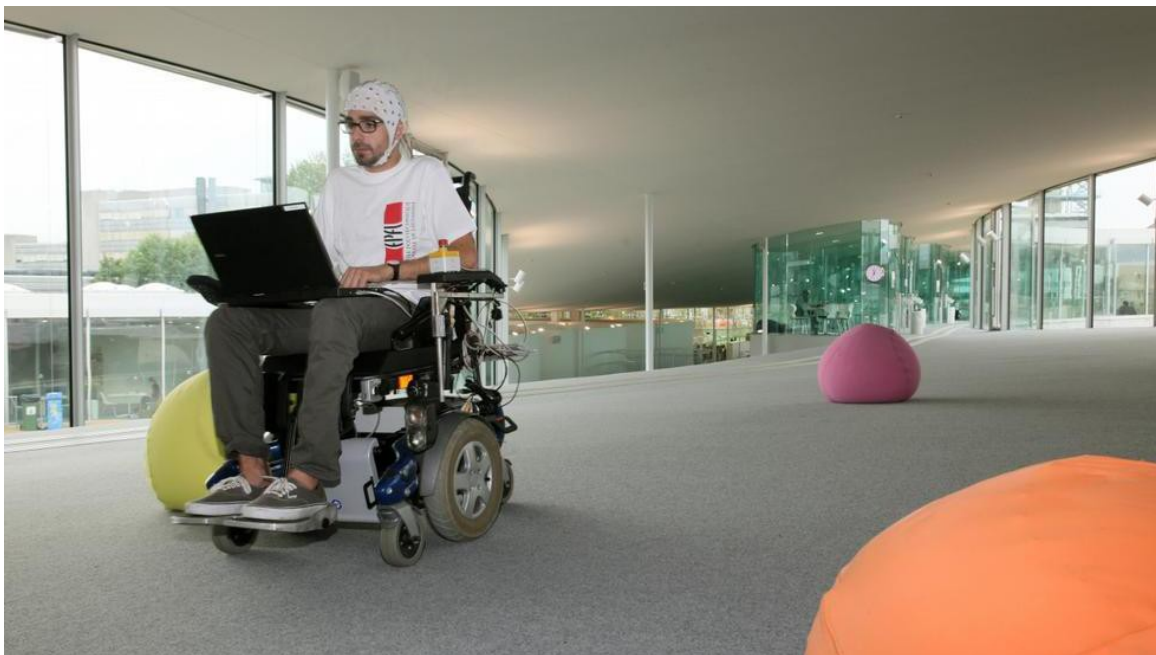
Figure 1.1: Controlling a wheelchair using motor imagery (picture from EPFL)
