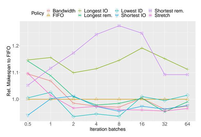
Figure III.6: Relative Makespan to FIFO of the different policies when varying the number of iteration batches.
