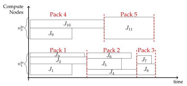
(a) The mapping of 11 applications into packs for two I/O nodes
