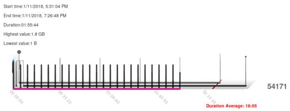
Figure I.3: Roughly periodical I/O behavior of an application, obtained from data provided by ATOS
