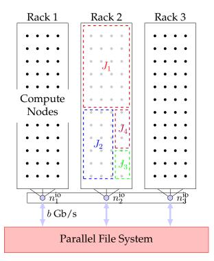
Figure III.2: Schematic of the architecture. Jobs  $J_1$ ,  $J_2$ ,  $J_3$  and  $J_4$  compete for the bandwidth available on  $n_2^{io}$ .
