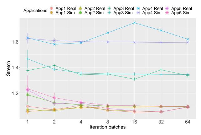
Figure III.7: Comparison of Simulated vs real execution (on the Tucan Machine) of the Longest I/O policy
