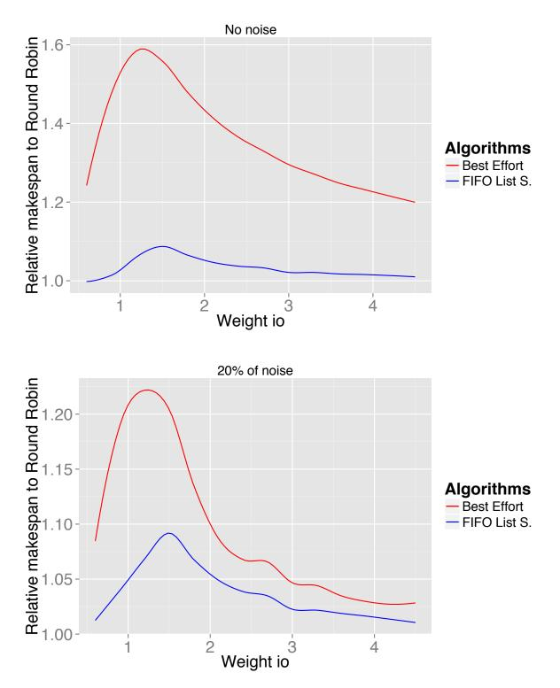
Figure II.6: Policies performance comparison of the ML use case for the makespan relative to HIERARCHICAL ROUND-ROBIN (top no noise, bottom 20% of uniform noise).
