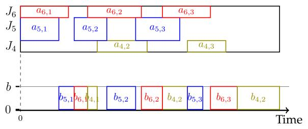
(b) The scheduling of I/O operations (bottom) within Pack 2. Computations are allocated on dedicated compute nodes and can start as soon as the I/O is transferred, but I/O operation share the available bandwidth b and can delay applications.
