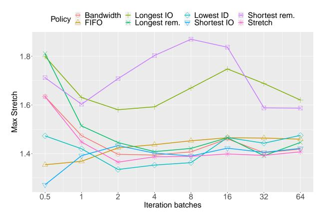
Figure III.5: Max Stretch of the different policies when varying the number of iteration batches.
