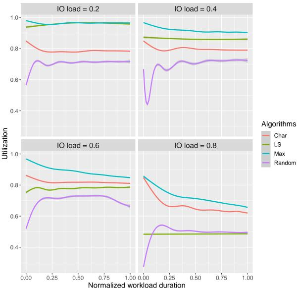
BU workload: Utilization depending on I/O load
