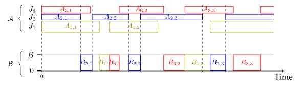
Figure II.1: Schematic overview of three jobs  $J_1$ ,  $J_2$ ,  $J_3$  scheduled on a bi-colored platform.
