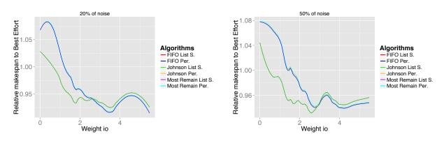
Figure II.5: Policies performance comparison on generic inputs for the makespan relative to the Best effort strategy with uniform noise on the computation or I/O duration
