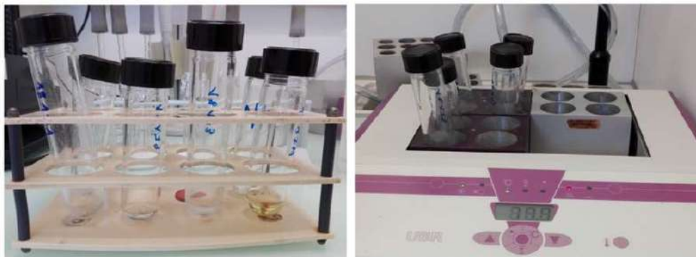
Figure 39. AAA chemical protocol classically applied on wood and charcoal ; HCl 0.5 M at room temperature (left) ; hot rinsing at 80 °C of the samples in glass tubes (right) (van Klinken and Hedges, 1998)
