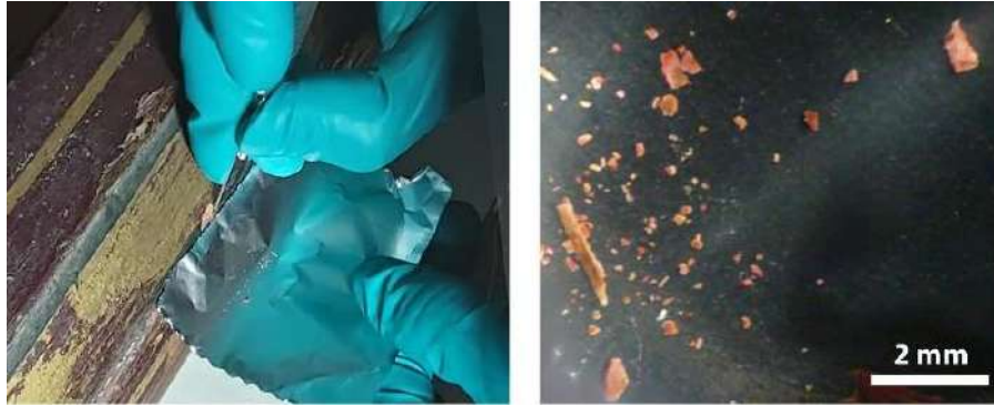
Figure 74. (left) The sample MGD127 with the dark red and the pink preparation layers taken on the left runner of the dragon sled (CMV64-1), (right) picture of the sample under binocular microscope (GifA20343).
