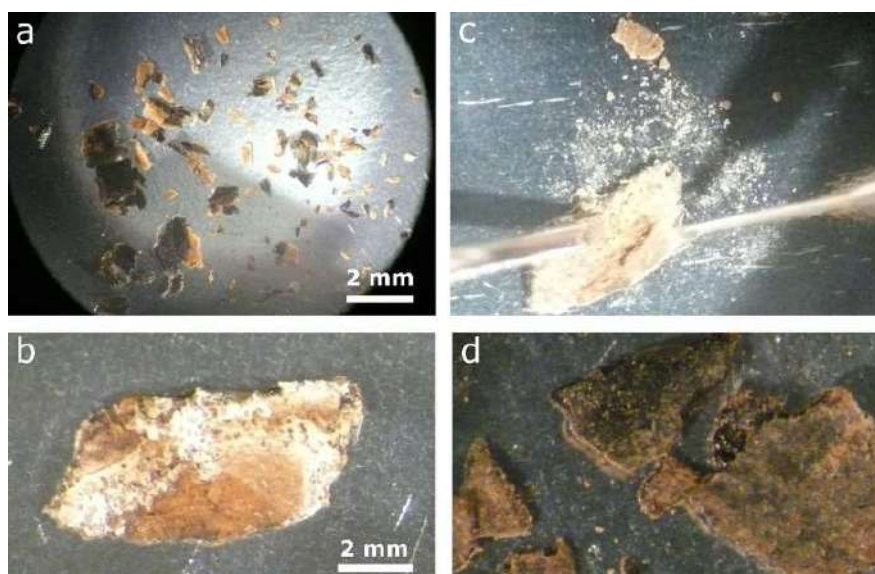
Figure 61. a) Chips of the MGD124 sample of Chinese lacquer with black and brown layers visible using a binocular microscope, b) the MGD125 sample of Japanese lacquer with an underlying white glue, c) mechanical abrasion of the brown lower layer of the Japanese lacquer sample MGD125, d) black upper layer of the Japanese sample MGD125.
