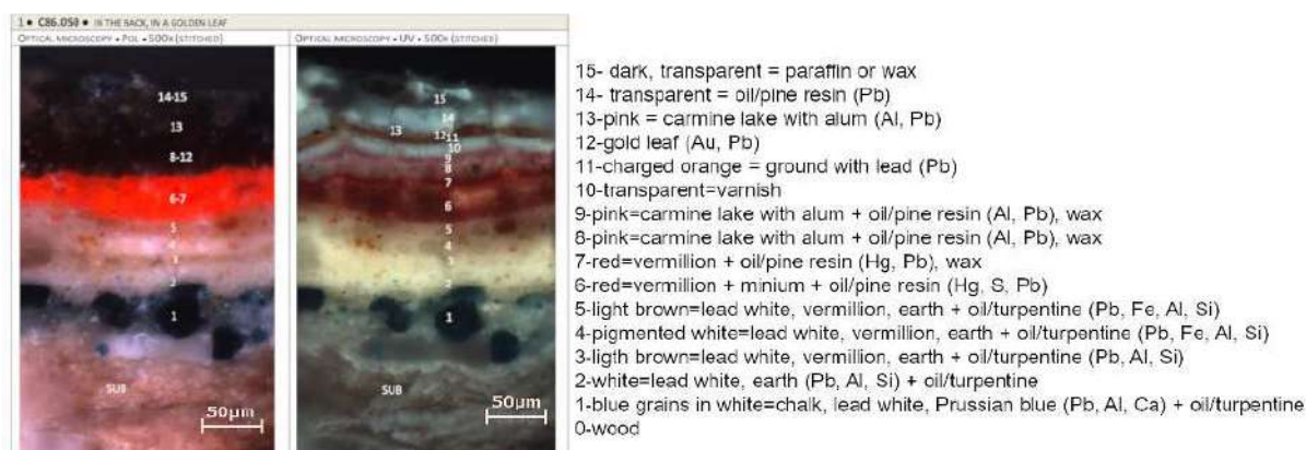
Figure 87. Stratigraphy performed by Louise Decq KIK-IRPA (figure adapted from unpublished report, KIK-IRPA, KMKG-MRAH © ElinC project) – Red and gold sledTR1868 (© KIK-IRPA / RMAH-KMKG, Brussels)
