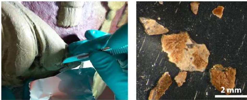
Figure 75. (left) The golden sample MGD128 taken on the left back side of the body of the dragon sled (CMV64-3), (right) picture of the sample under binocular microscope (GifA20344).
