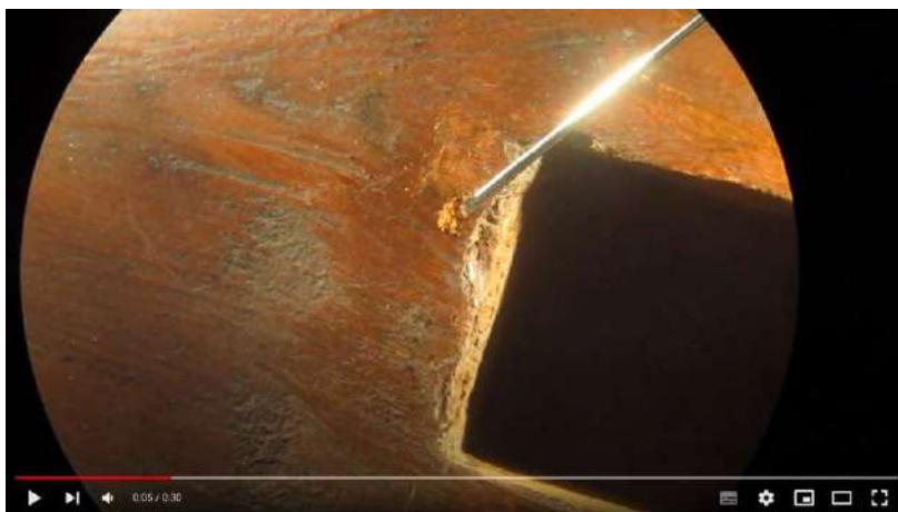
Figure 37. Sampling of red lacquer on a Chinese qin D.04224 at the Musée de la musique, Paris. Sample and video taken by Marie-Gabrielle Durier. https://youtu.be/izfl40391ck
