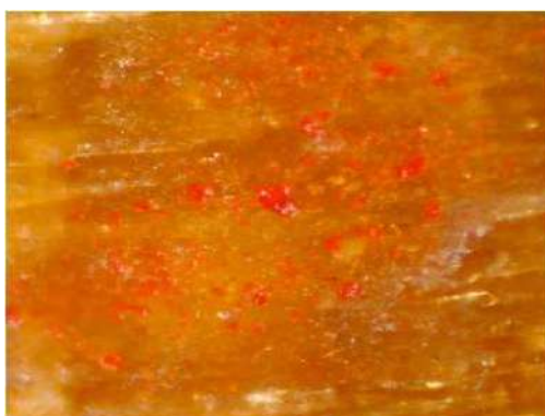
Figure 26. Optical image of the varnish of the "Sarasate", violin, Stradivari, Cremona, 1724, Musée de la Musique, E.1729, with scattered vermilion grains (Echard, 2010)
