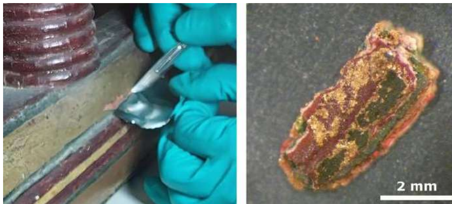
Figure 73. (left) The red and gilded sample MGD126 taken without the preparation layer on the left runner of the dragon sled (CMV64-1), (right) picture of the sample under binocular microscope (GifA20342)
