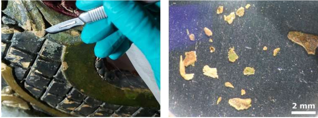
Figure 69. (left) The green and gilded sample MGD130 taken without the preparation layer on the right side of the body of the eagle sled (CMV57.006-1), (right) picture of the sample under binocular microscope (GifA20346)
