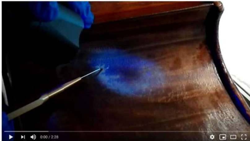
Figure 36. Varnish sampling on a cello, Namy, 1773, Paris, private collection using a microchisel 0.5 mm under UV light performed by Sebastiaan Kirsh. Video taken by Marie-Gabrielle Durier https://youtu.be/Neen31VA8DQ
