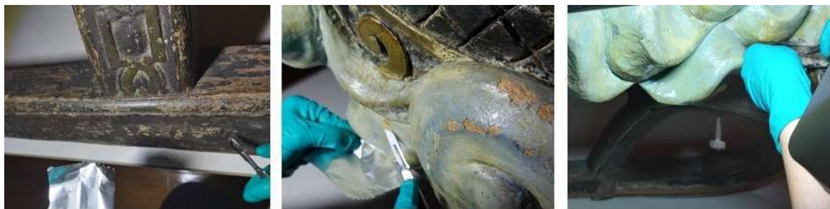
Figure 70. (from left to right) green sample MGD131 from the right runner (CMV57.006-2), the pale blue sample MGD132 under the cloud body (CMV57.006-3), sample MGD133 of the boiled oil applied in the 1960s, taken from the cloud body (CMV57.006-4)
