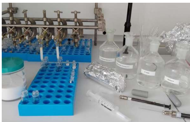
Figure 122. Application of the Geosh protocols to separate molecular fractions according to increasing polarity (cyclohexanes, alcohols, alkenes, aromatic molecules, etc.).
