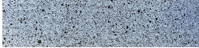
Figure 39: Image to show the hand-sprayed speckle pattern on the tensile specimen.
