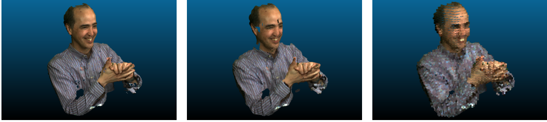
Figure 3.4: Original point cloud (left), the compressed point cloud using the proposed method (middle) and the MPEG anchor (right). Colors are mapped using nearest neighbor matching. Our compressed point cloud was compressed using \lambda = 10^{-6} with a PSNR of 29.22 dB and 0.071 bpov. The anchor compressed point cloud was compressed using a depth 6 octree with a PSNR of 23.98 dB and 0.058 bpov. They respectively have 370,798; 1,302,027; and 5,963 points.
