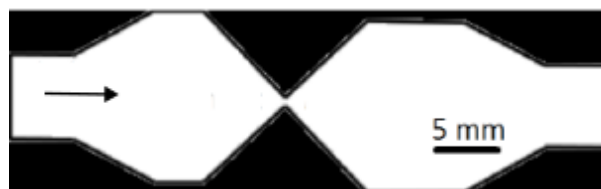
Figure 2.2: Typical mask provided by SELBA. The white area allows the passage of U.V. rays to activate the resin following the desired shape. Black areas obstruct the passage of the light and covered zones remain inactivated.
