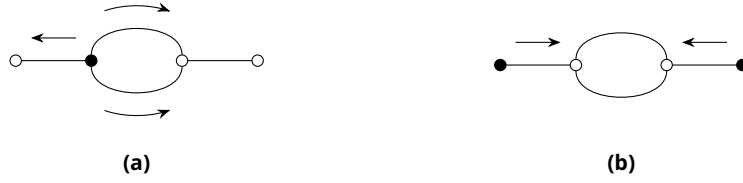
Figure 12: Diagram (a) is inconsistent because all the energy is flowing out of the loop. On the other hand, in (b) all the energy is flowing into the loop.
