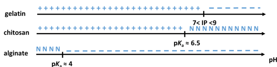
Figure 2 – Summary of the state of charge (+ : positive; - : negative; N : neutral) of gelatin, chitosan and alginate in function of pH
