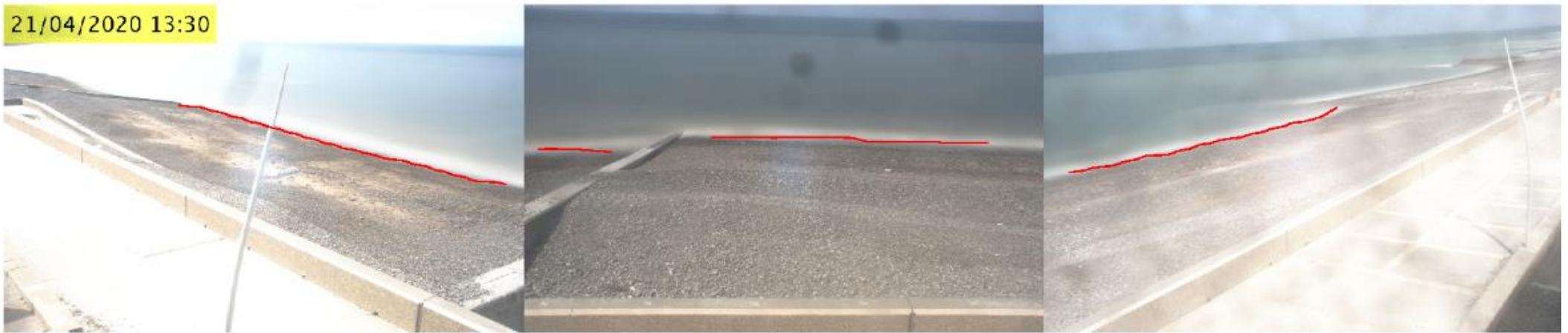
Figure 50 - Example detected waterlines on the 3 cameras of the Hautot-sur-Mer's VMS
