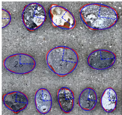
Figure 33 - Comparison between sediment particles' shape as detected with Mask R-CNN (red) and the ellipse fitted around this shape (blue). The ellipses' major and minor axes are displayed as dashed blue lines.
