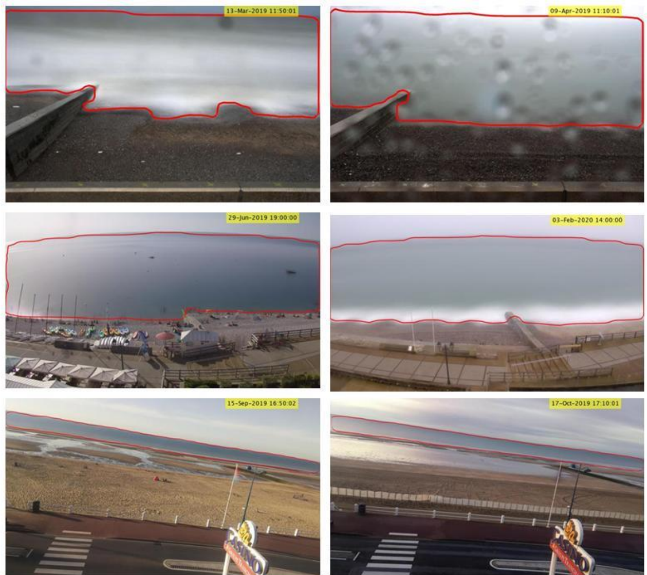
Figure 49 - Example of body of water detection using Mask R-CNN in Hautot-sur-Mer (top), Etretat (center) and Villers-sur-Mer (bottom), during various filming conditions
