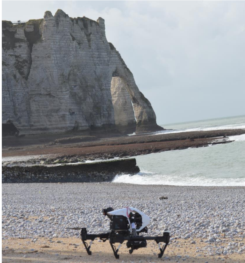
Figure 30 - UAV used for mapping the pebble beaches of Normandy
