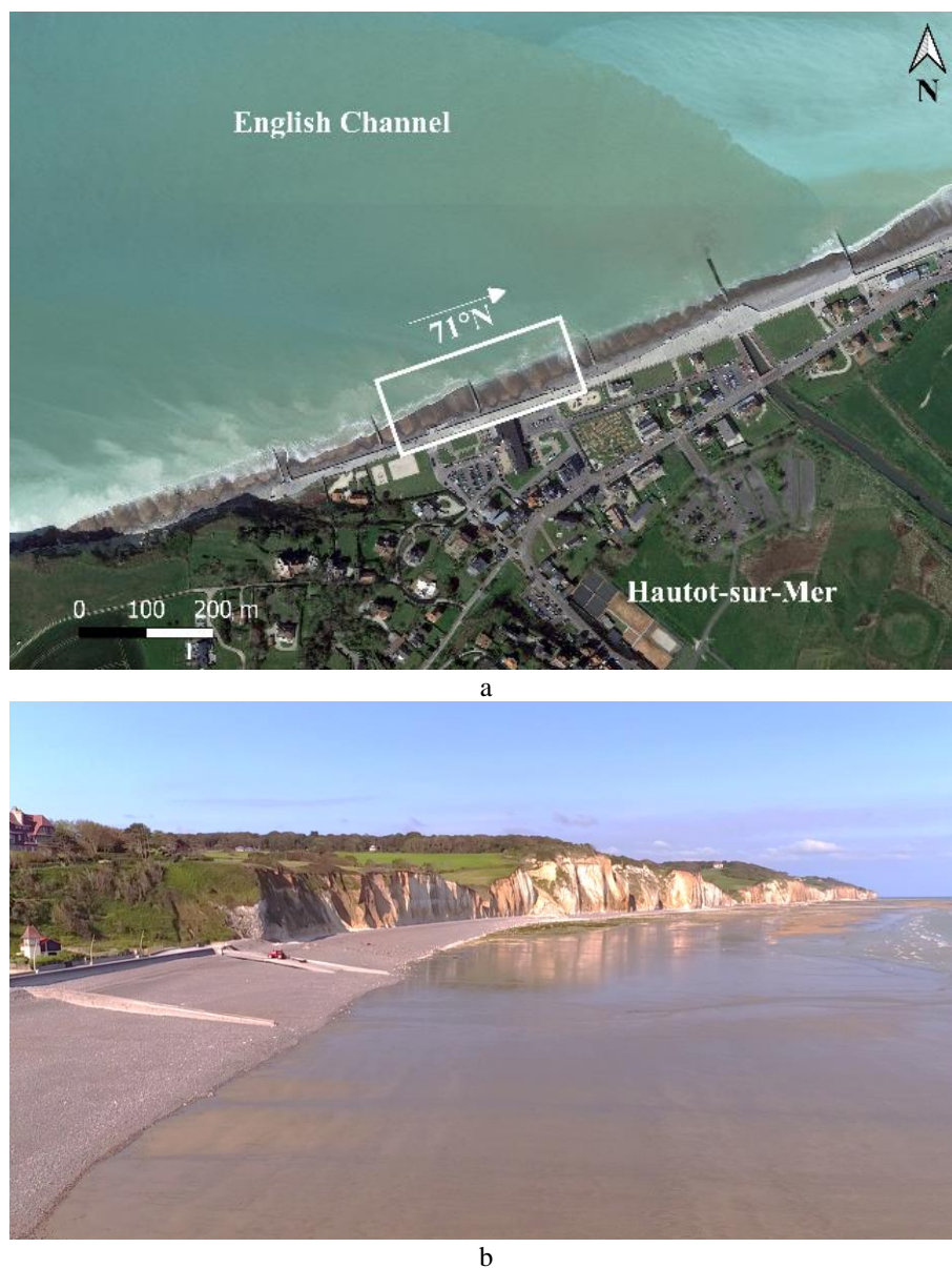
Figure 23 – a: Satellite photography of Hautot-sur-Mer, the white rectangle indicates the area monitored with VMS; b: aerial cross-shore view of the beach including the pebble ridge and coastal defense structures (left), and the sandy low tide terrace (center). The image was taken at low tide using a drone (credit: P. Rouxin, 2019).
