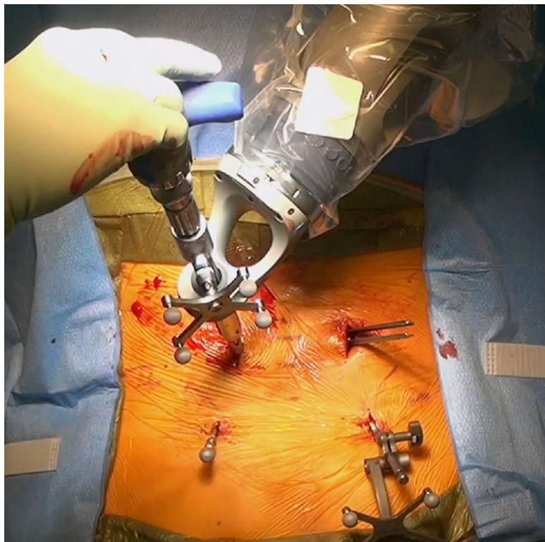
FIGURE 1.13: Robotically-assisted minimally invasive pedicle screw placement [Farber et al., 2021].
