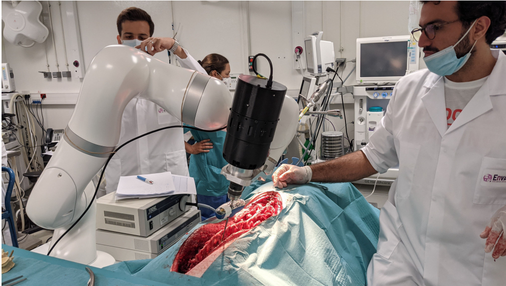
FIGURE 4.17: Experimental setup at the veterinary school to test automatic drillings with Algorithm 3 and the threaded drill bit on a living pig.
