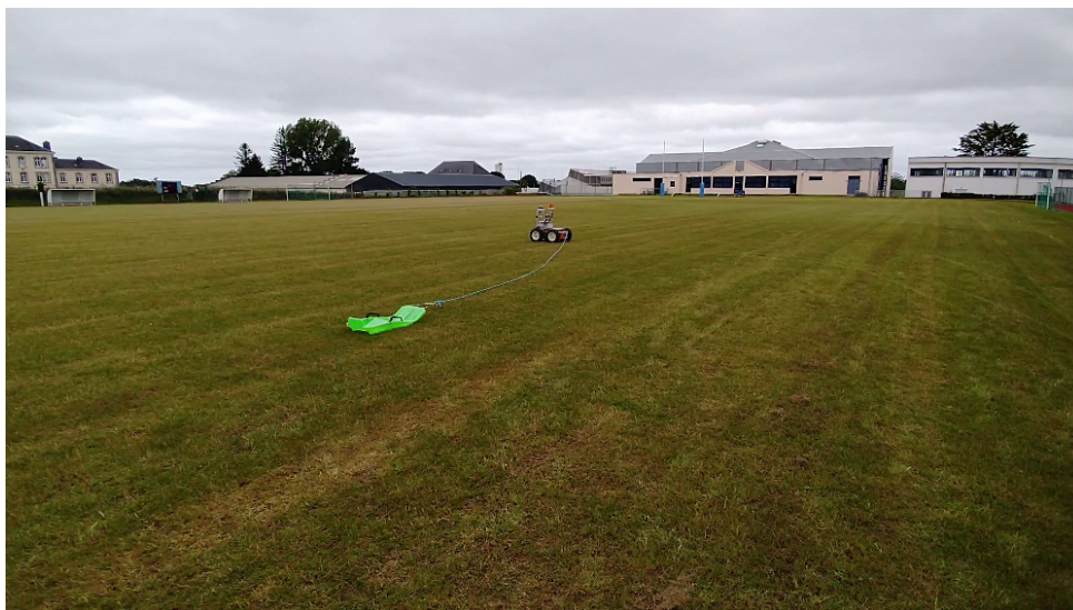
Figure 3.11: The green sled is towed by Saturne , an Unmanned Ground Vehicle (UGV).
