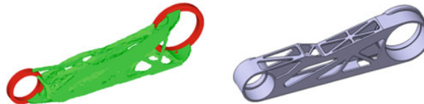
Figure 1.13: Topology optimization of the upper frame of a painting robot (Kim et al., 2016).
