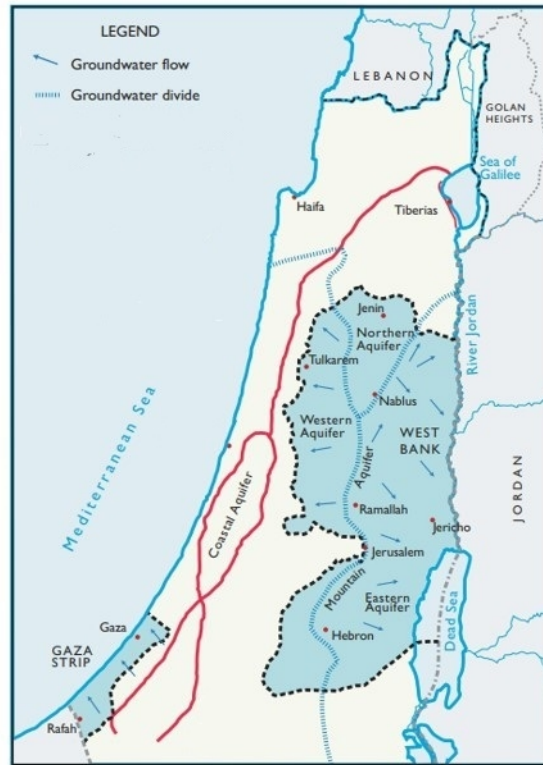
Figure 2.3. Groundwater flow, divides and aquifers in the West Bank and Gaza Strip
