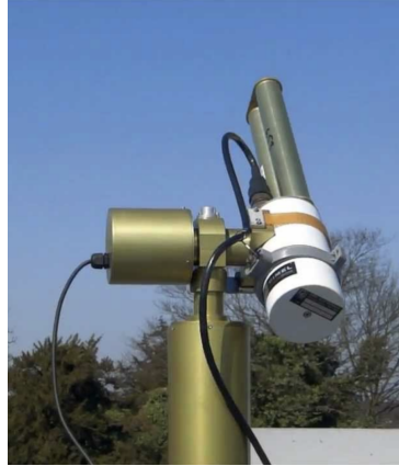
Figure 2.1: CIMEL sunphotometer set up during a sky measurement where the robot arm and the optical head can be appreciated. Photography source: GOA-UVa.
