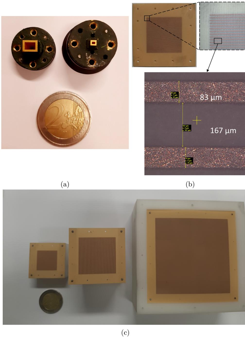
Figure 4.7: (a) Photograph of the employed pyramidal horns. Model 32240-10 is shown on the right and model 32240-20 is shown on the left. (b) Close-up view of one of the fabricated transmitarrays. (c) Photograph of the three employed sizes of the four transmitarrays. Prototypes A and B exhibit the same size, shown on the left. Prototype C is shown on the right and prototype D in the middle.
