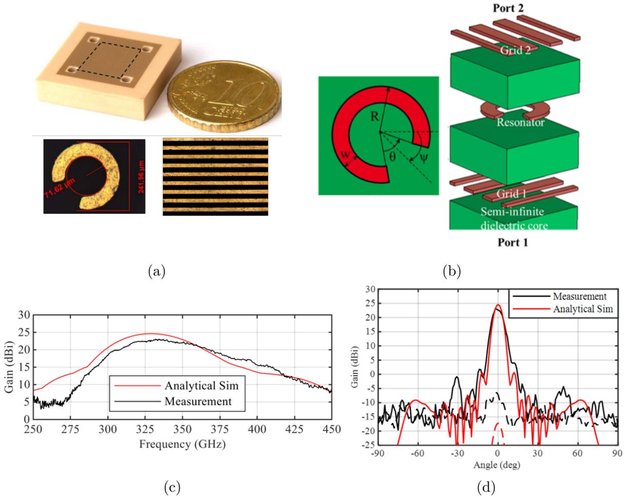
Figure 1.17: (a) Photograph of the prototype reported in [48], showing one rotator unit-cell and the top grid. (b) Geometry of the three-layer unit-cell. (c) Measured and simulated gain versus frequency of the prototype. (d) Measured and simulated E-plane radiation pattern at 332 GHz.
