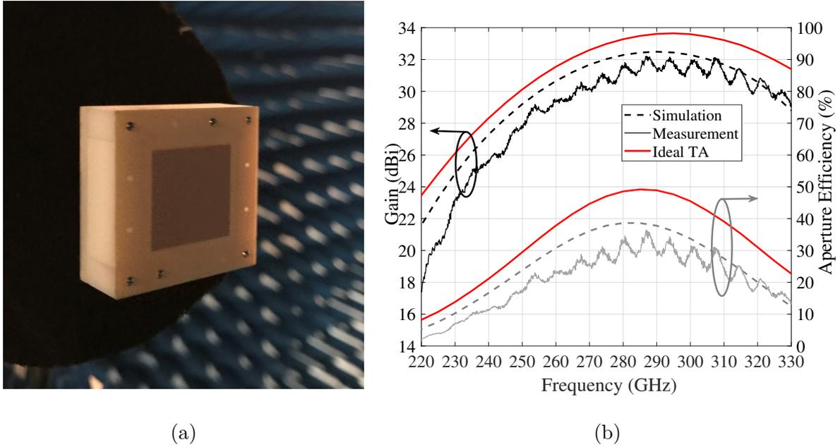
Figure 4.15: (a) View of prototype B. (b) Simulated and measured results of the gain and aperture efficiency as a function of frequency. The red curve depicts the gain and aperture efficiency of an ideal transmitarray on the same setup, which can be used as a reference for maximum performance.
