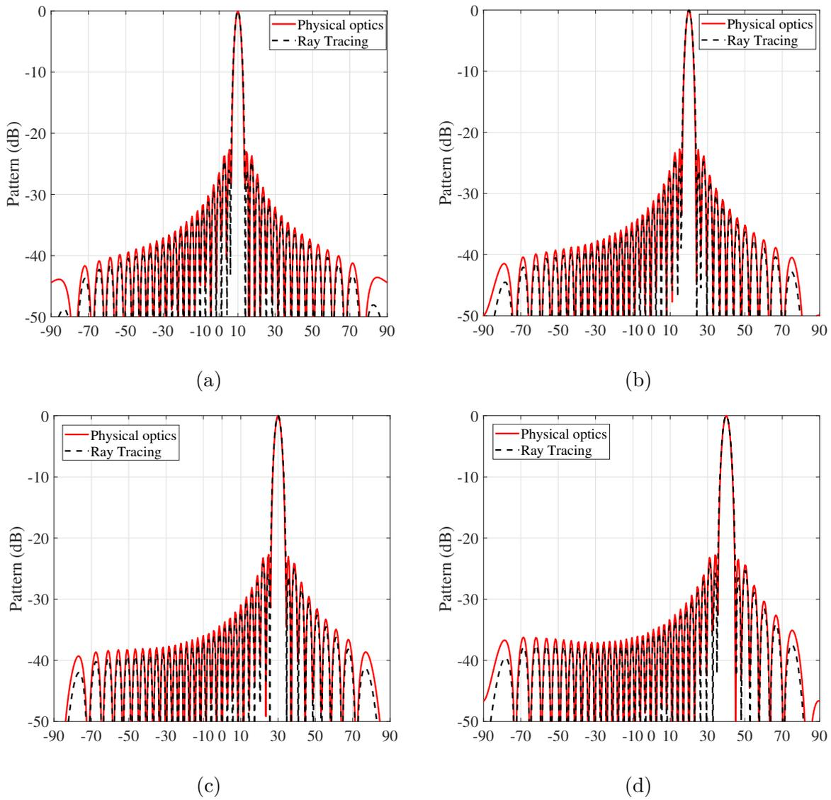
Figure 2.10: Radiation pattern of a theoretical transmitarray calculated using the two discussed techniques for (a)  $\theta_0 = 10^\circ$ , (b)  $\theta_0 = 20^\circ$ , (c)  $\theta_0 = 30^\circ$  and (d)  $\theta_0 = 40^\circ$ , while  $\phi_0 = 0^\circ$  in all cases.
