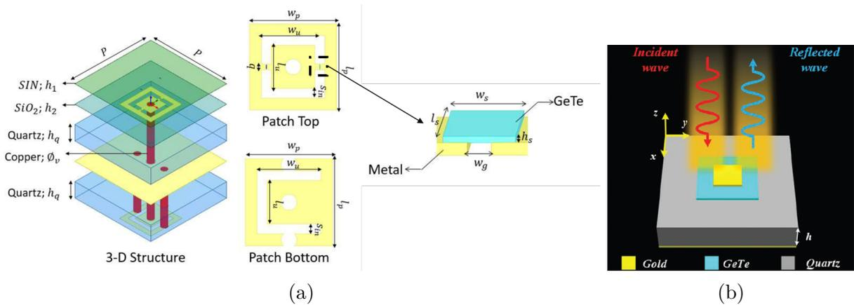
Figure 1.25: Unit-cell topology integrating patterned GeTe used as a PCM for (a) a transmitarray [71] and (b) a reflectarray [72] design.
