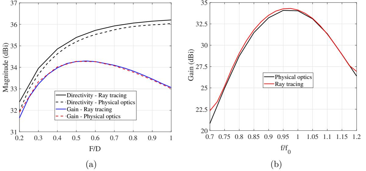
Figure 2.7: Comparison of the peak gain as a function of (a) the focal distance at  $f_0$  and (b) the frequency when  $F/D = 0.55$  between the ray tracing and the physical optics approach, using the 10 dBi Flann horn as a focal source.
