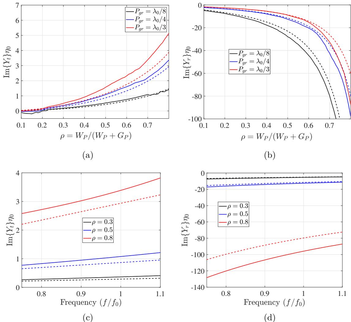
Figure 3.3: Simulated (solid lines) and numerical (dashed lines) normalized admittances  $Y_t$  and  $Y_r$  using (3.3) of a polarizer that is interleaved between vacuum and some dielectric with relative permittivity  $\epsilon_r = 4$ . The values in (a) and (b) are plotted as a function of the filling factor at  $f_0$  and those in (c), (d) are plotted as a function of the frequency for  $P_{gr} = \lambda_0/4$ .
