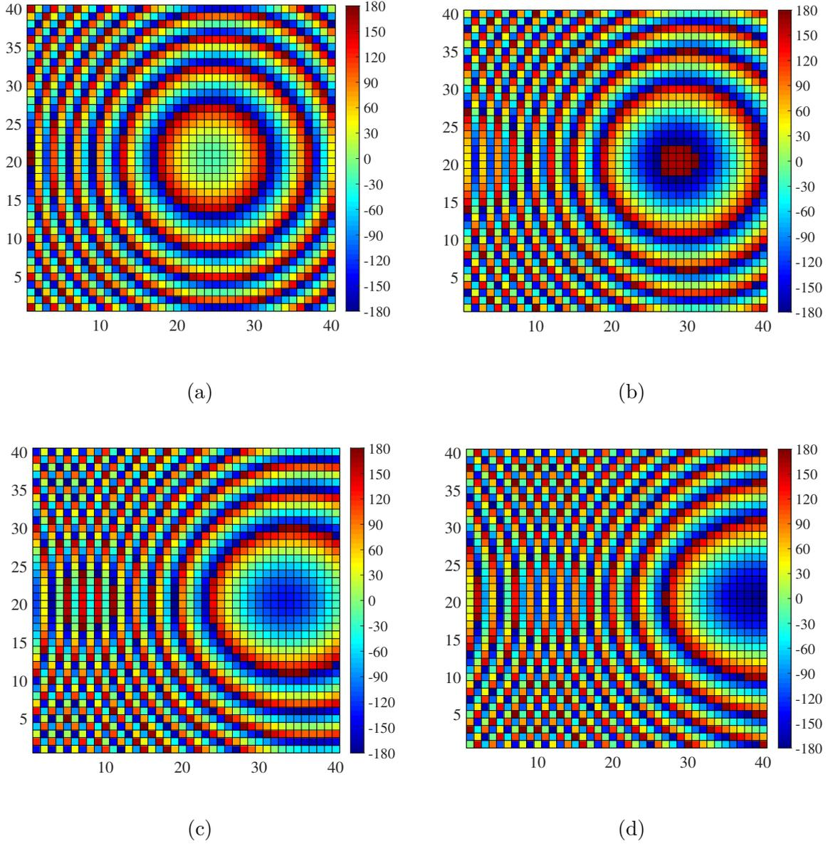
Figure 2.11: Corresponding phase distribution of the transmitarray for the steering angles depicted in Figure 2.10. (a)  $\theta_0 = 10^\circ$ , (b)  $\theta_0 = 20^\circ$ , (c)  $\theta_0 = 30^\circ$  and (d)  $\theta_0 = 40^\circ$ , while  $\phi_0 = 0^\circ$  in all cases.
