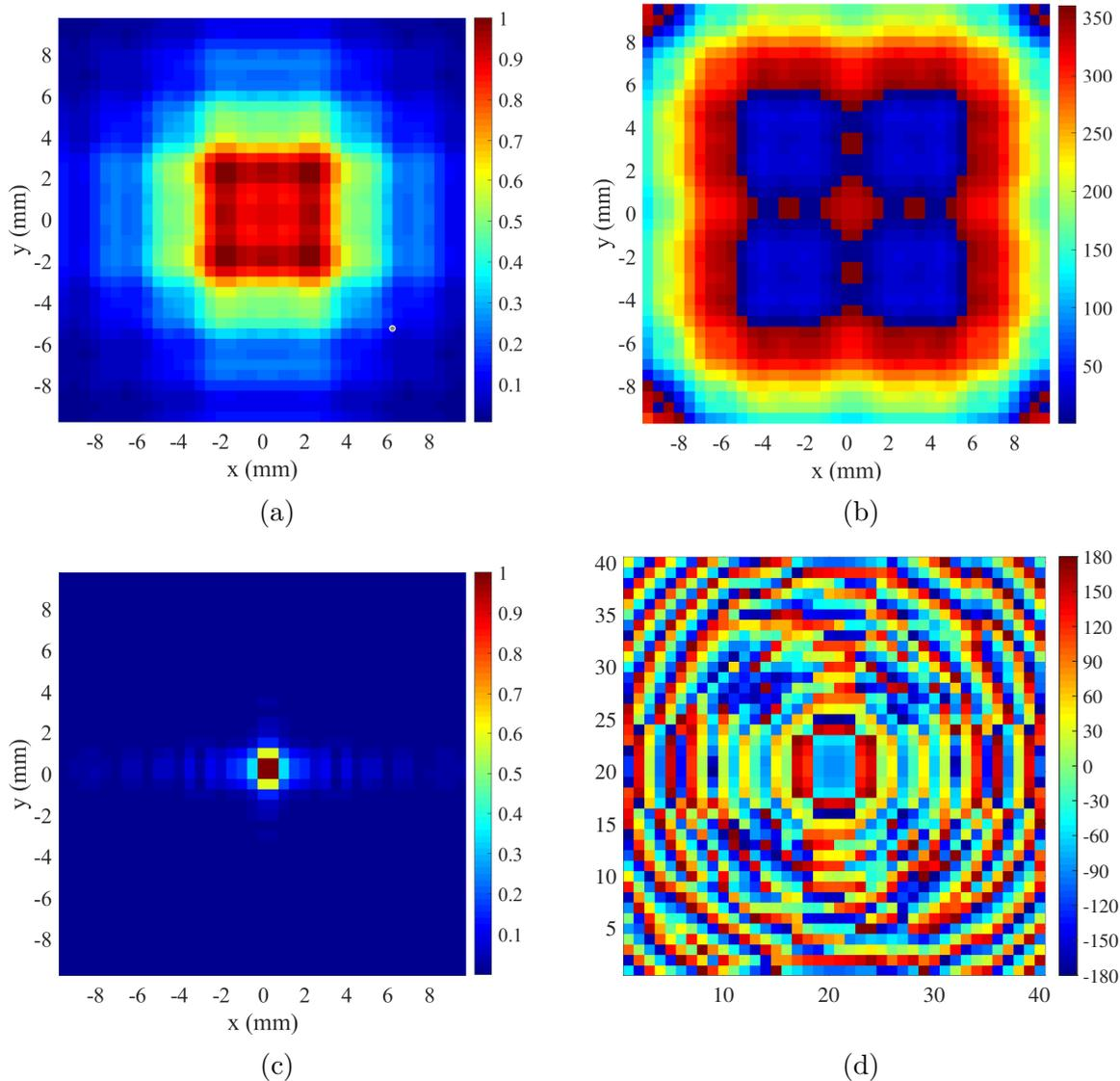
Figure 2.13: (a) Normalized amplitude and (b) phase (deg) of  $x$  component of the incident field on the transmitarray using the physical optics technique. (c) Normalized amplitude and (d) phase (deg) of the incident field on the  $40 \times 40$ -elements transmitarray using the ray tracing technique. In both cases the selected  $F/D$  is equal to 1.
