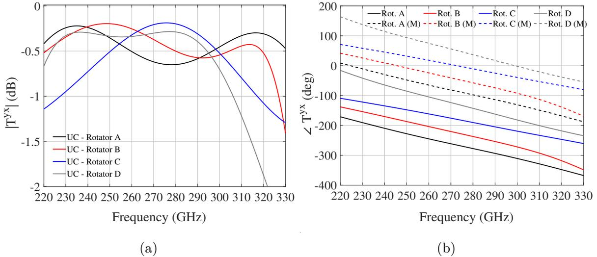
Figure 4.3: Transmission magnitude (a) and phase (b) of the designed unit-cells, obtained from full-wave simulations. The results when the rotators are mirrored (M) with respect to  $x$ -axis are shown in dashed lines.
