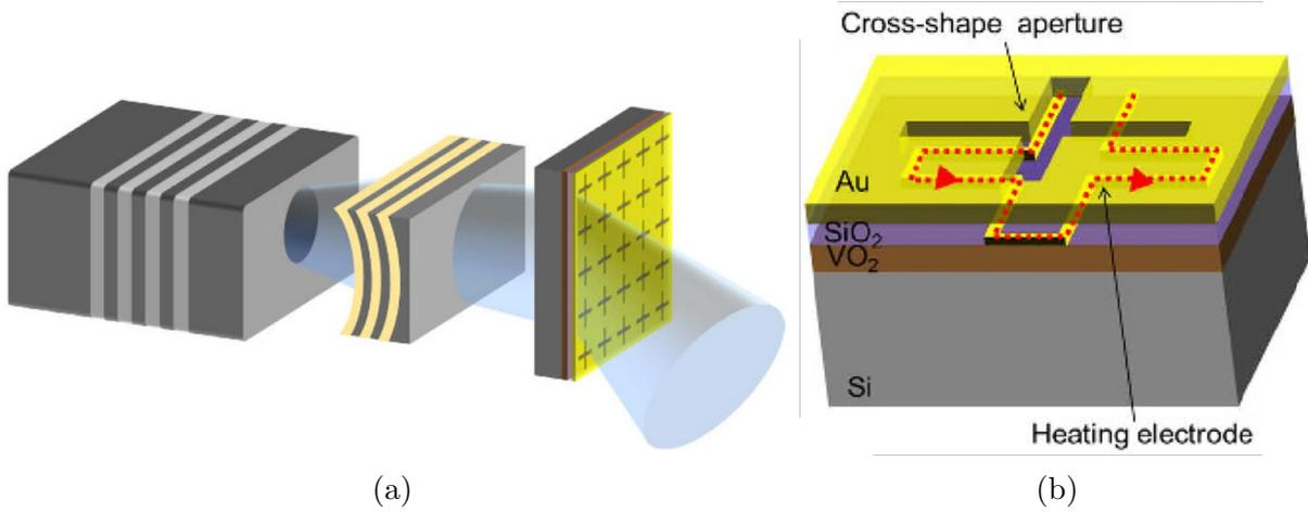
Figure 1.24: (a) Beam-steering metasurface system using a vertical external cavity surface emitting laser, reported in [67] (b) Metasurface unit-cell comprising VO<sub>2</sub> for a PCM.
