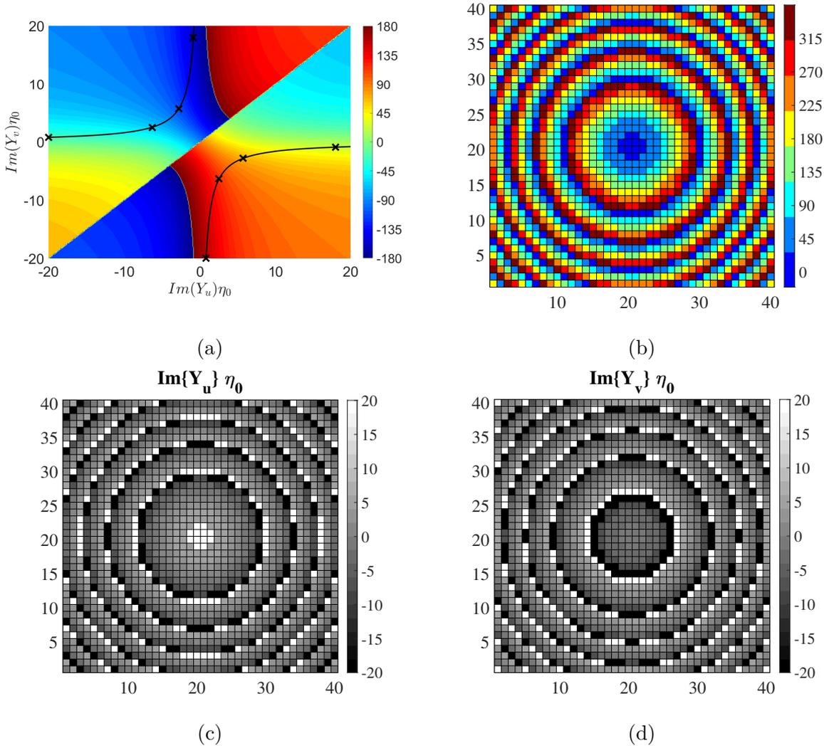
Figure 3.9: (a) Phase of transmission as a function of the admittance pair  $(Y_u, Y_v)$  at 300 GHz, including the locus for maximum transmission (-0.25 dB) and the solution points for a 3-bit TA design, marked with crosses. (b) Phase distribution of a 3-bit TA for broadside radiation. (c), (d) Admittance map of the rotator calculated at the crystal axes, based on the results shown in (a).
