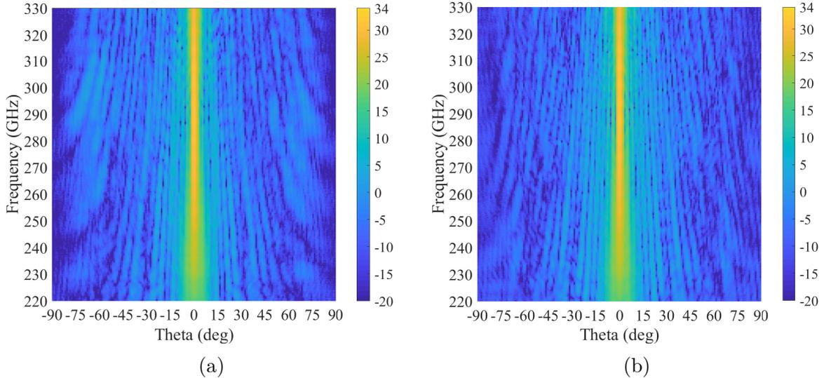
Figure 4.16: Measured gain of prototype B as a function of elevation angle and frequency in (a) H- and (b) E-plane.
