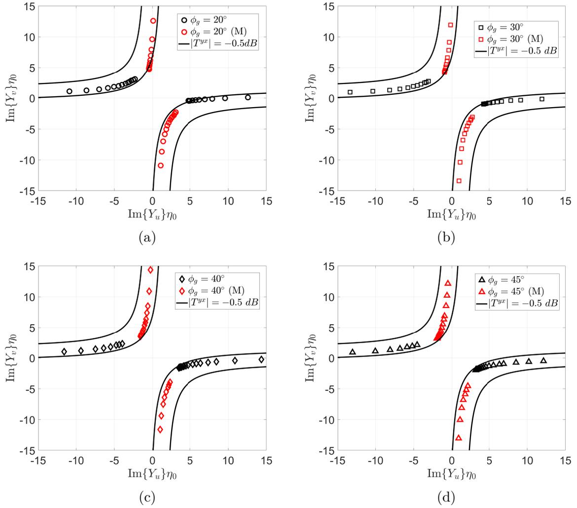
Figure 5.2: Admittance properties in the crystal axes of the rotator in Figure 5.1(b) for different opening angles,  $\phi_g$ , when the offset angle  $\phi_{off}$  varies from  $0^\circ$  to  $60^\circ$ . Most admittance pairs fall in the region where  $|T^{yx}| \leq 0.5$  dB, highlighted by the two loci (dark solid curves) at each graph. The results when the rotator is mirrored (M) are depicted with red symbols.
