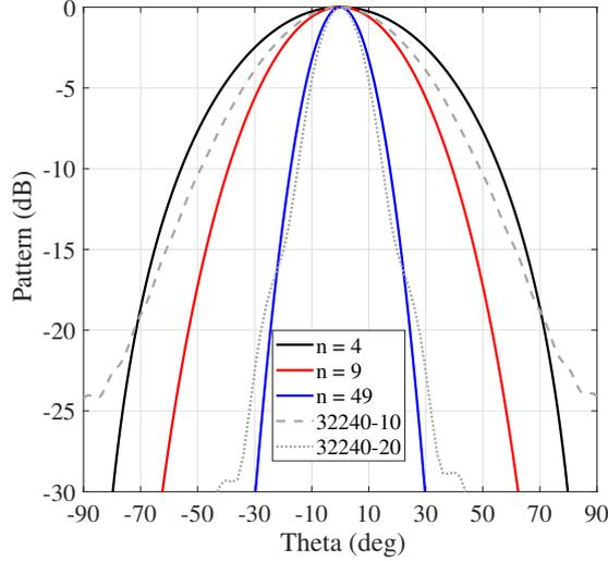
Figure 2.3: Radiation pattern of the theoretical cosine source for different values of index  $n$ , along with the two employed pyramidal horns in the E-plane.
