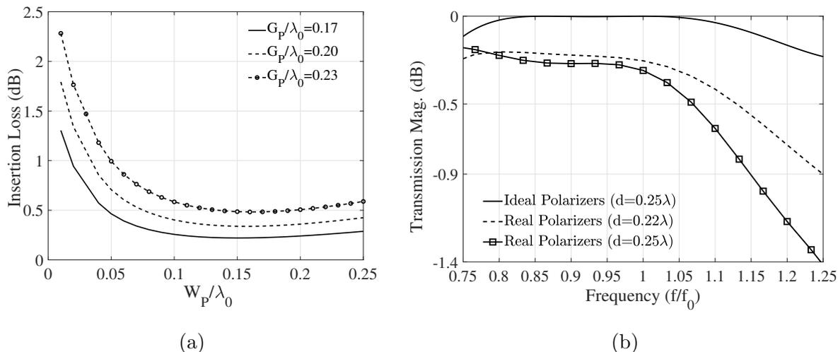
Figure 3.8: (a) Minimum insertion loss of the unit-cell as a function of the strip width,  $W_P$ , for three gap values,  $G_P$ . (b) Transmission coefficient (magnitude) as a function of frequency considering ideal and real polarizers.
