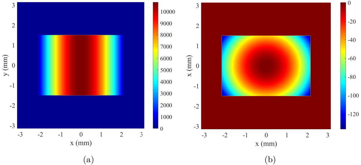
Figure 2.6: Field distribution of horn Flann 32240-10, calculated numerically using expressions (2.28).
