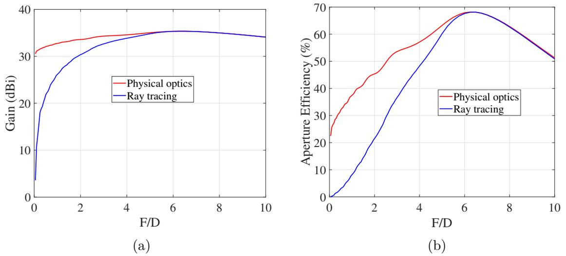
Figure 2.12: Comparison of the gain (a) and the aperture efficiency (b) as a function of the focal distance, between the ray tracing and the physical optics approach. The transmitarray has a size of  $20 \times 20 \lambda^2$  and it is illuminated by a square-shaped focal aperture with size of  $10 \times 10 \lambda^2$ .
