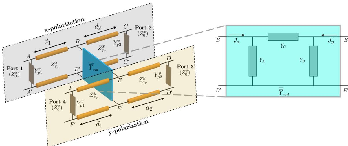
Figure 3.2: Equivalent four-port circuit of the unit-cell. Both polarizers,  $p_1$  and  $p_2$ , are represented as a pair of shunt admittances at the ends of  $x$  and  $y$  transmission lines, respectively. The rotator is modelled by a  $\pi$ -type network, coupling the two transmission lines at  $BB'$  and  $EE'$ .
