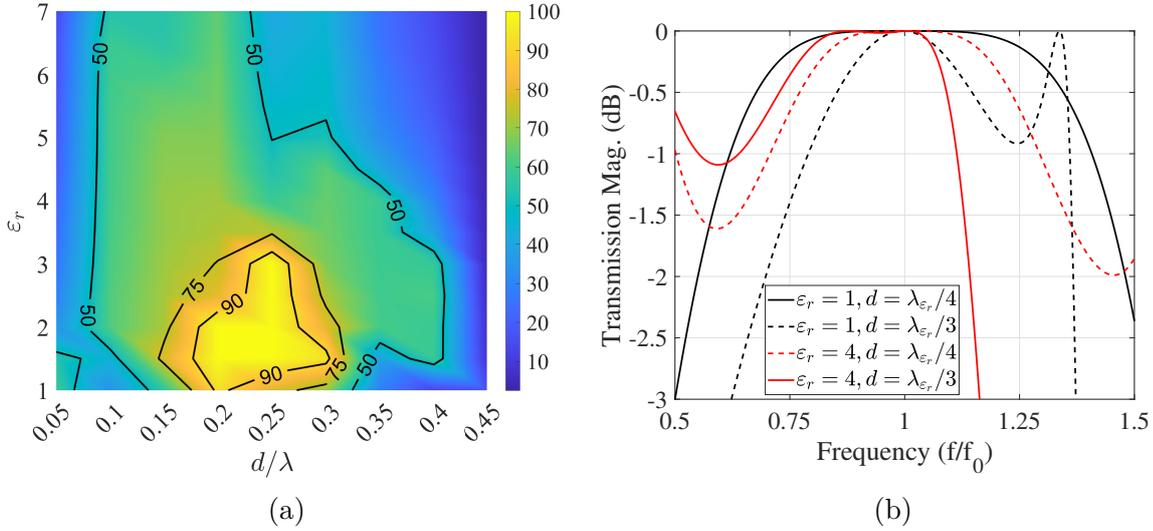
Figure 3.7: (a) 1-dB relative bandwidth (in %) of the unit-cell as a function of thickness and permittivity of the spacers, assuming ideal polarizers. (b) Transmission coefficient (magnitude) for different values of permittivity and thickness as a function of frequency.
