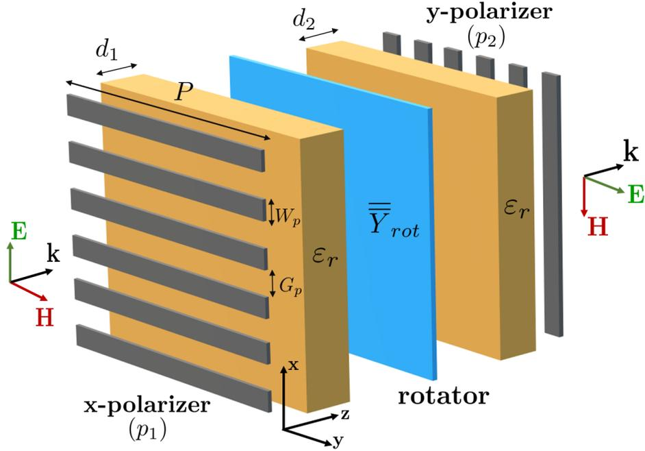
Figure 3.1: Exploded view of the ALP unit-cell with  $P$  periodicity, which is the same along the  $x$ - and  $y$ -axis. The rotator (blue color) is generically modelled as a two-dimensional sheet impedance described by a  $2 \times 2$  admittance matrix. The polarization grids (grey color) are orthogonally oriented. The layers are interleaved by two dielectric spacers (orange color) of the same permittivity,  $\varepsilon_r$ .
