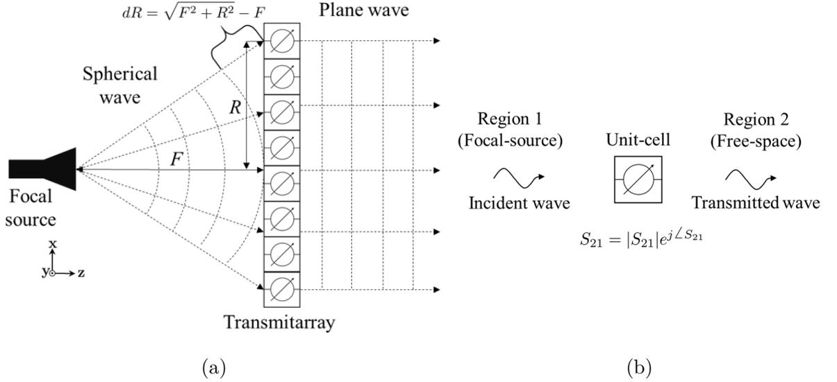
Figure 1.12: (a) Operating principle of the transmitarray antenna, (b) transmitarray unit-cell.
