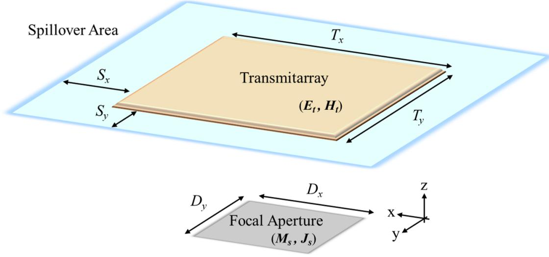
Figure 2.5: Geometry for the calculation of the transmitted field using physical optics.
