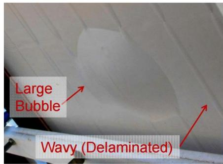
*Fig. III.5: Backsheet/encapsulation fault [22]*
