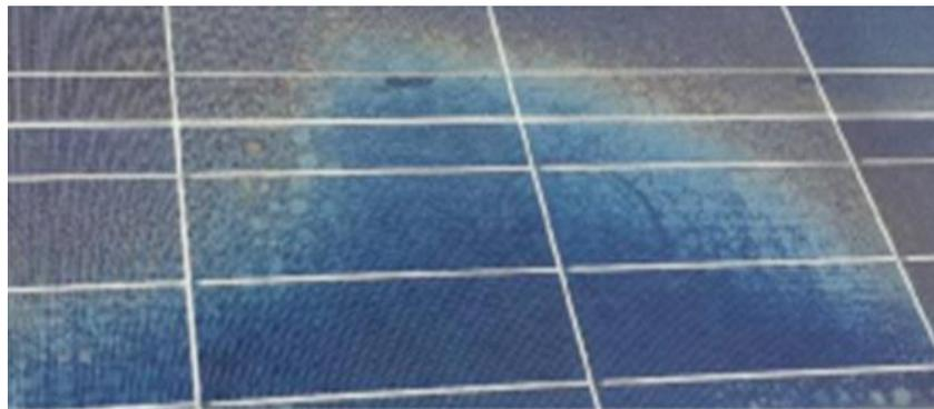
*Fig. III.6: Bubbles in a PV module [14]*
