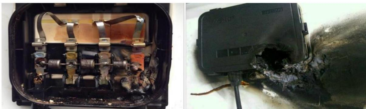
*Fig.III.10: Junction box failure [14]*
