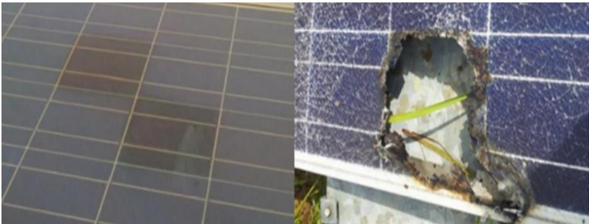
Fig.III.8: PV module with hot spot [14]
