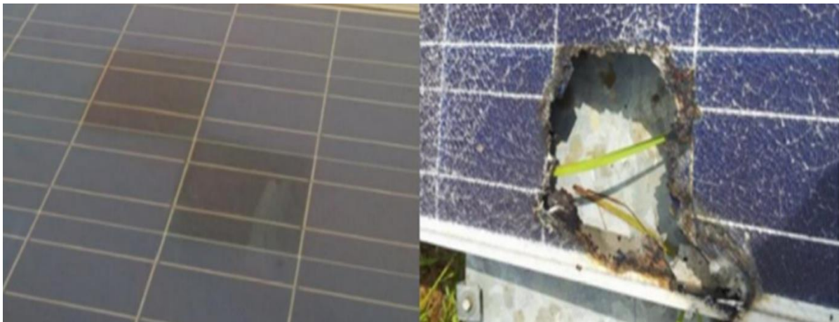
Fig.III.8: PV module with hot spot [14]
