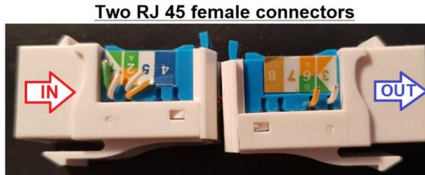
Figure 3.9 Data Diode unidirectional physical link
