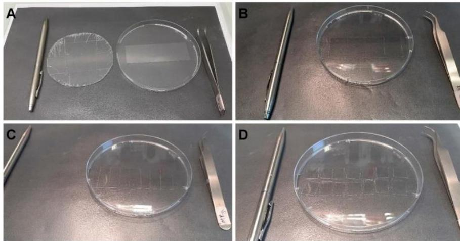
**Figure 2. Cutting coated slides.** A. From left to right, diamond pencil, plastic to avoid breaking, Petri dish containing silane-PEG-biotin slide, tweezers. B. The slide is cut in four equal parts. C. A silane-PEG slide is cut in 7 parts. D. Each part is cut in half.
