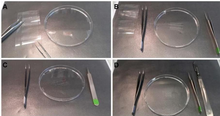
**Figure 3. Construction of the flow chamber.** A. One piece of silane-PEG-biotin is put in a Petri dish. B. Adhesive tape is stuck to the slide. C. Protective plastic above the tape is removed and one piece of silane-PEG slide is placed onto the tape. D. Excessive tape is cut and removed.
