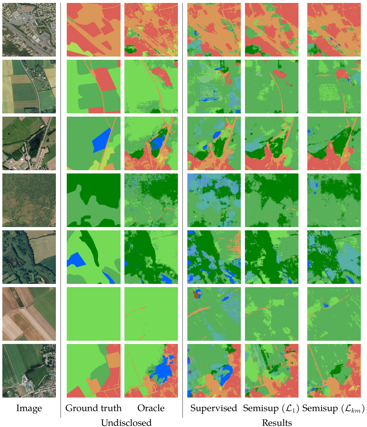
Figure 3.3 – Classification examples of different methods over tinyMiniFrance. Oracle refers to the hypothetical case where all ground-truths are available for training regions (8 annotated training cities). Supervised refers to the results of a network trained only on the labeled training split of tinyMiniFrance, while semi-supervised corresponds to the BerundaNet-late network trained over all available training data (labeled and unlabeled). SegNet architecture is used as backbone.
