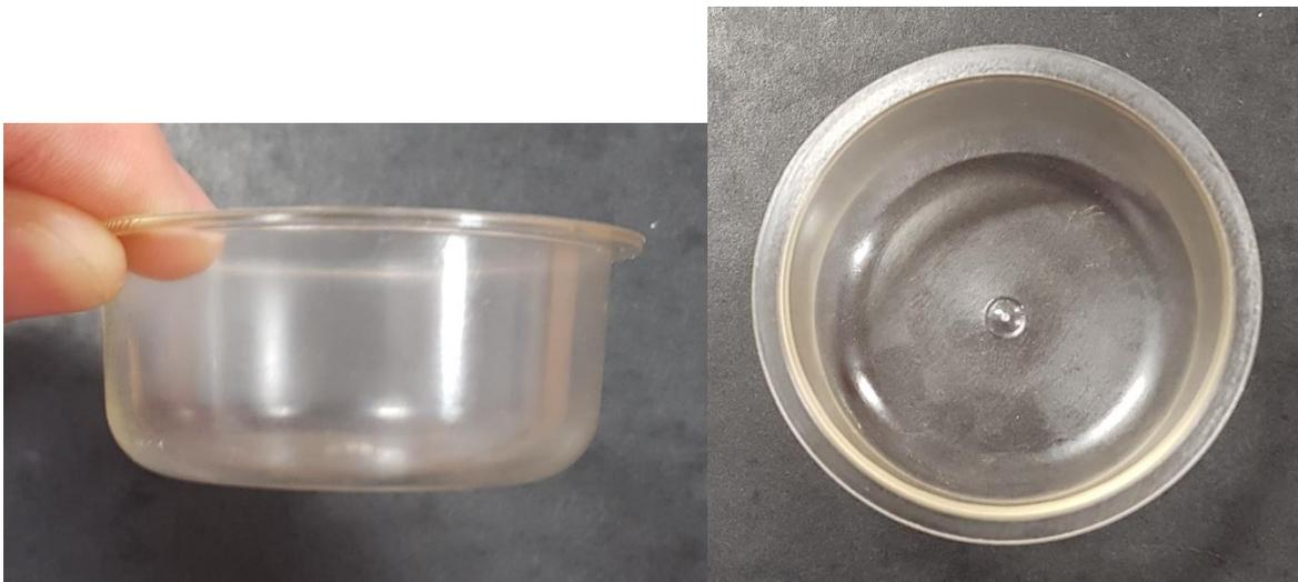
Fig III. 11: Picture of an injection moulded neat PLA cup
