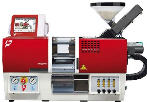
*Fig VI.3: Babyplast 6/12V injection moulding machine*
