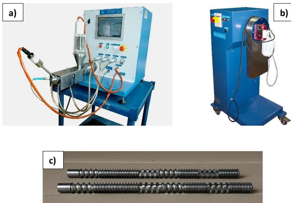
*Fig VI.2: a) Scamex extruder, b) Scamex pelletiser, c) Twin corotating screws*
