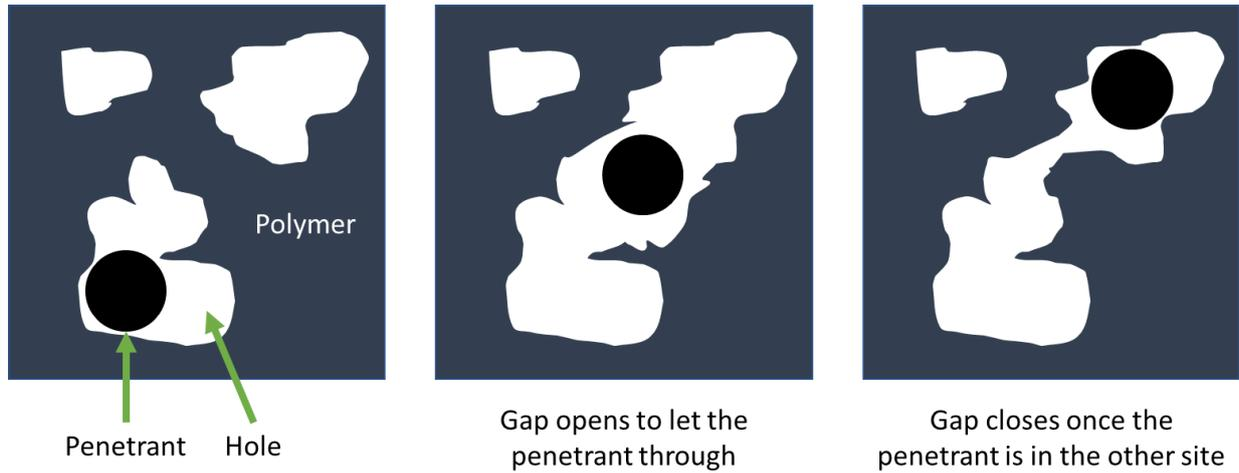
Fig. 1. 11: Schematic representation of the mechanism of the of a penetrant transport in a polymeric material
