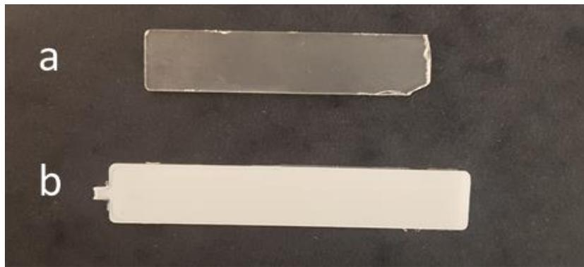
*Fig. II. 14: DMA samples of an injection moulded a) neat PLA, b) PLA + 1wt% Stear-C4 at 110°C for 75secs*
